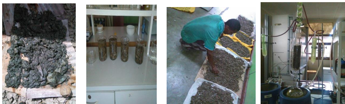
a/ fleshing waste b/waste soaked in 1% wt. /wt. boric acid c/ chopped dried waste d/oil extraction using Soxhlet
