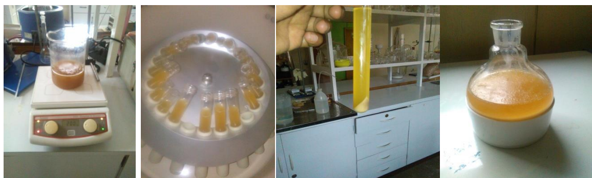
a/degumming b/ centrifuging c/gum and oil separation d/ storage of oil in moisture free container
