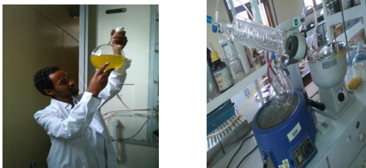
a/ oil and extractive b/ separation of oil and extractive using rota vapor
