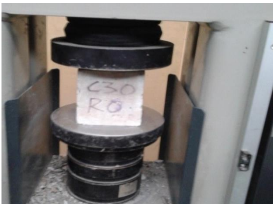
Compressive strength test
