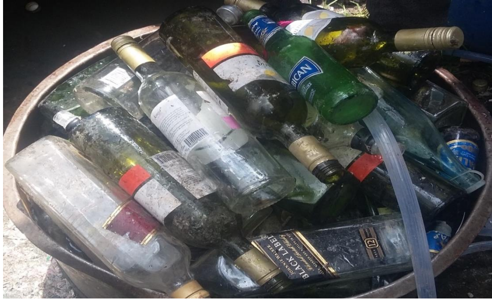
Figure 3-2 Cleaning waste glass
