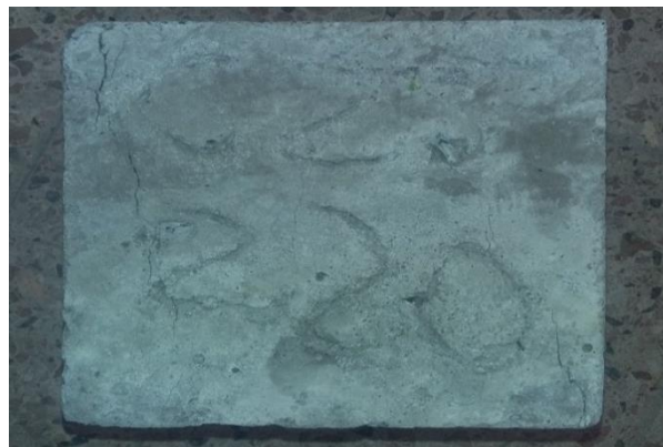
Concrte cube after compressive strength test
