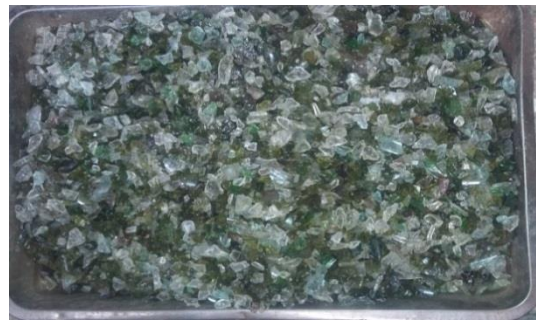
Crushed and sieved glass
