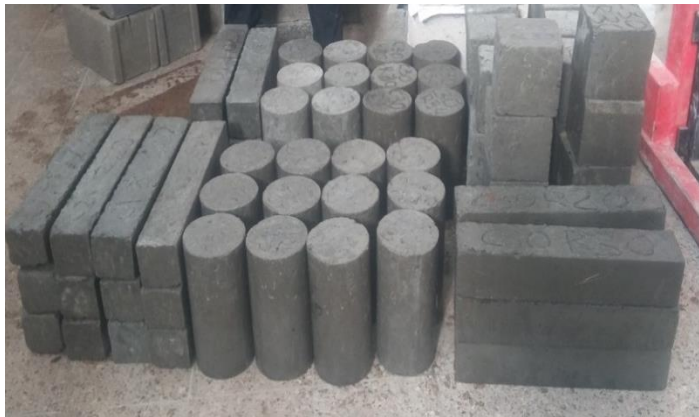
Hardened concretespecimens ready for test
