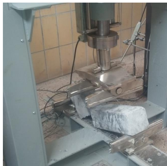
Crushed beam specimen
