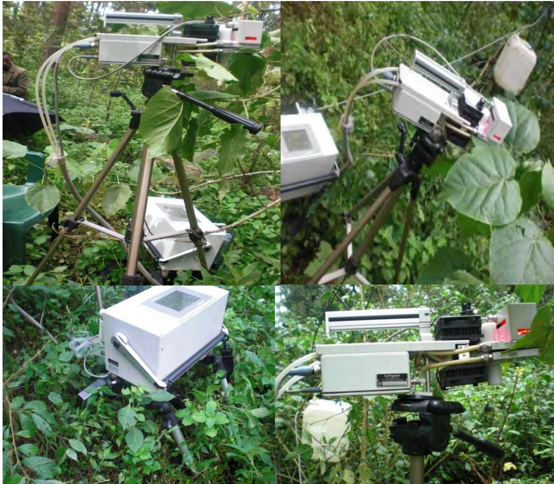
Fig 2.4.2 Porometer used to measure photosynthesis and dark respiration of the studied trees. Photo Y.S.
