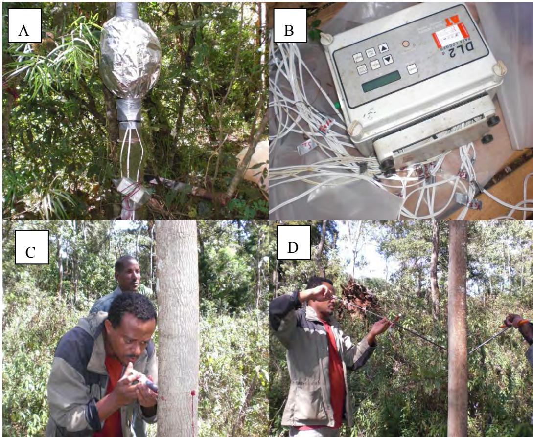
Fig 2.5.3 P. falcatus tree installed with Granier type sensors and wrapped with aluminum foil (A), sap flux DL2 datalogger (B), dye injection on C. macrostachyus tree (C) wood core samples being taken from injected tree of C. macrostachyus . Photo Y.S and Getu Teshome.
