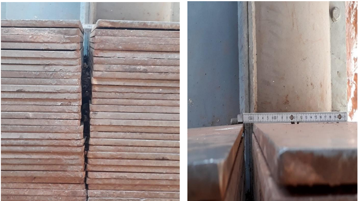
Figure 3.1.1-11:-Column-D3 (Bending of plates towards the column center and Slight uniform opening of plate is witnessed on this column)
