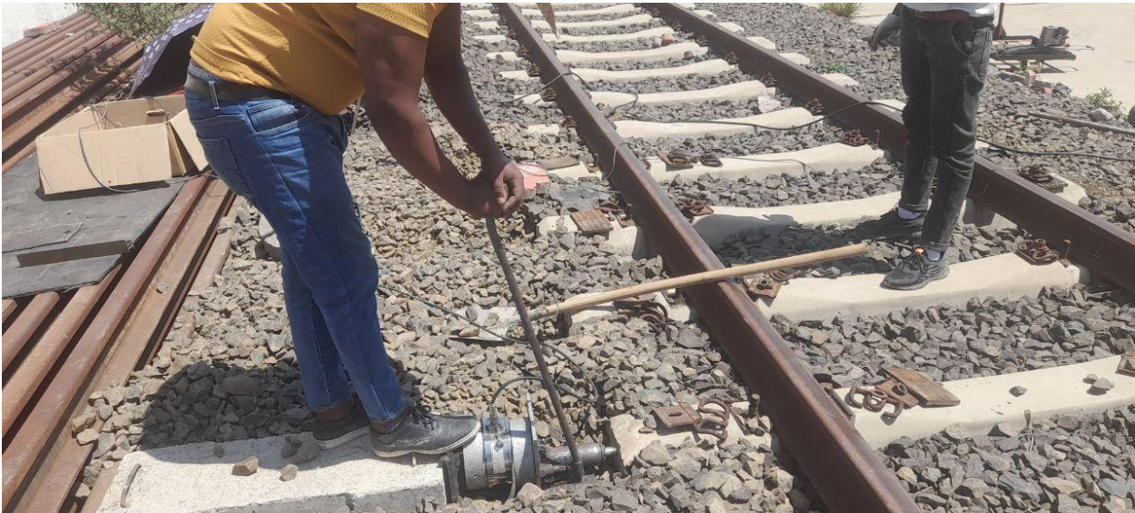
Figure 3.15: Lateral load applied to the tested sleeper
