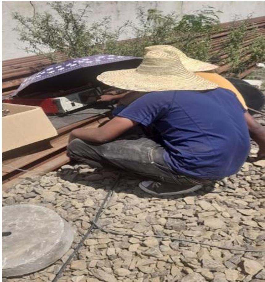
Figure 3.14: Installation and adjustments of the load and displacement reading setting on the data logger
