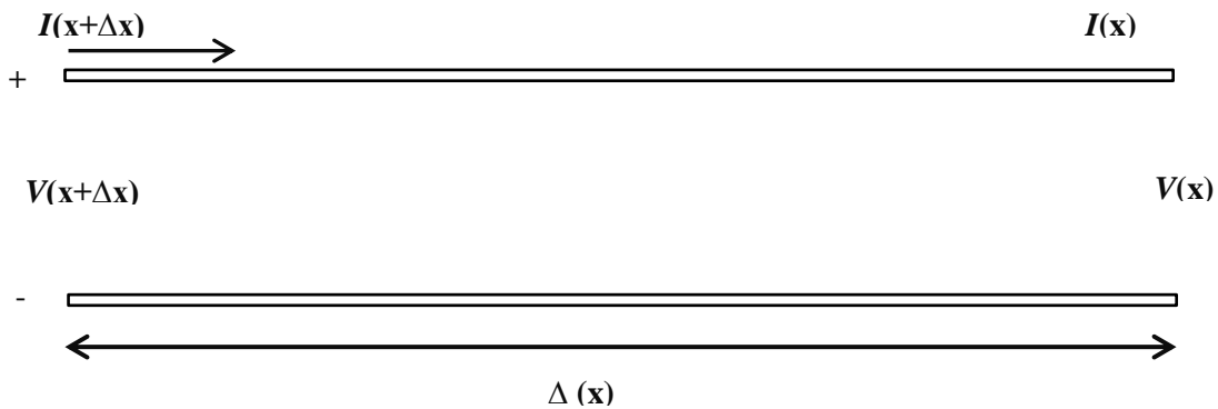
Fig 7: Simple Two-wire Transmission Line
