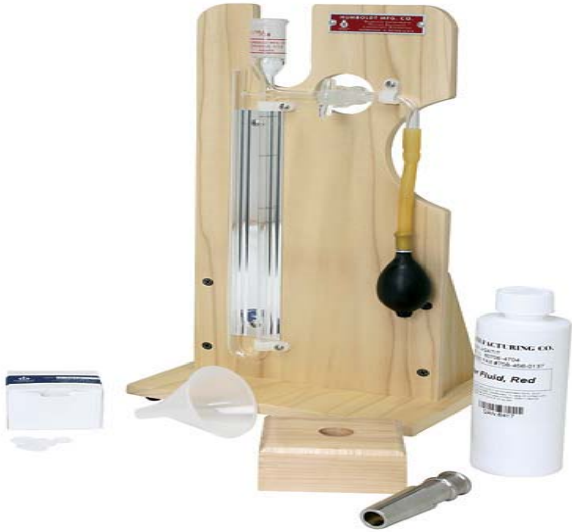
Fig 3.6 Set-up of Blaine air permeability apparatus
