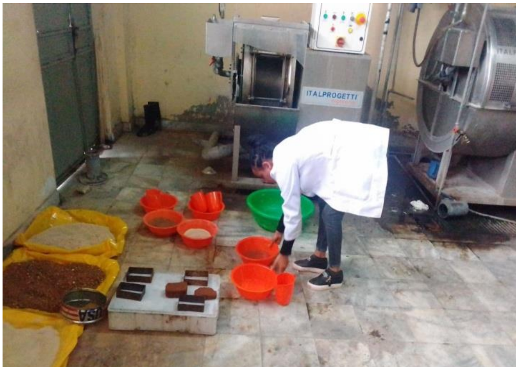
A. Weighing and preparing different proportion of white clay, red clay, and sludge
