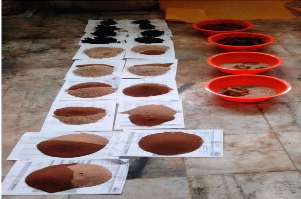
A. Weighing and preparing different proportion of white clay, red clay, and sludge
