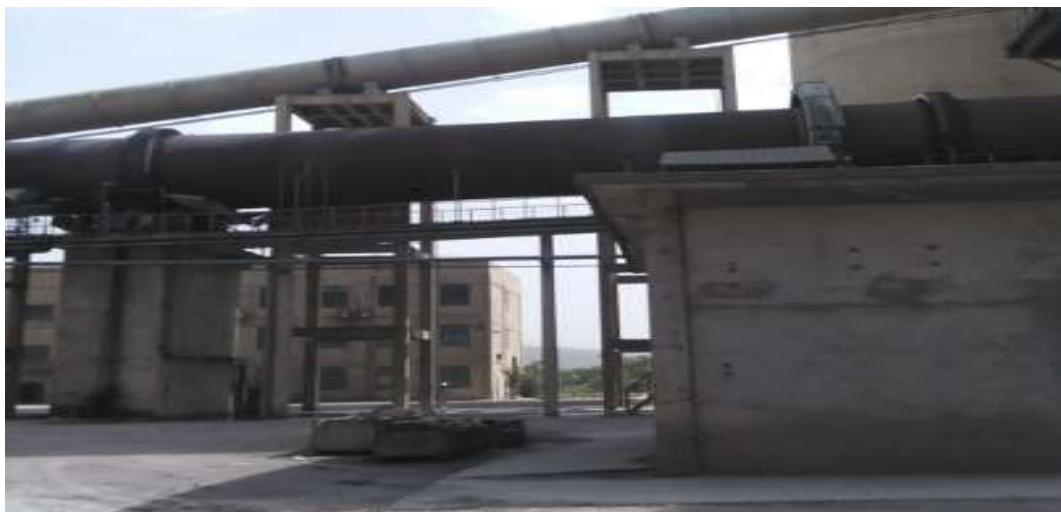
Figure 2.5 Production of Clinker [from Diredawa National Cement]
