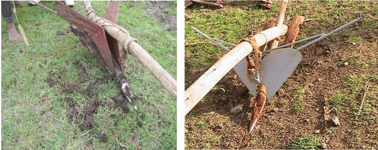
Figure 3. 2 The modified broad bed and furrow makers (BBM) used for this experiment
