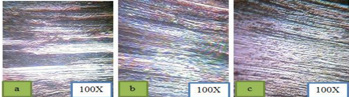
Figure 4-12 Microstructure at 400 0 c and (a) at 30min tempering time, (b) at 60min tempering time,(c) at 90min tempering time
