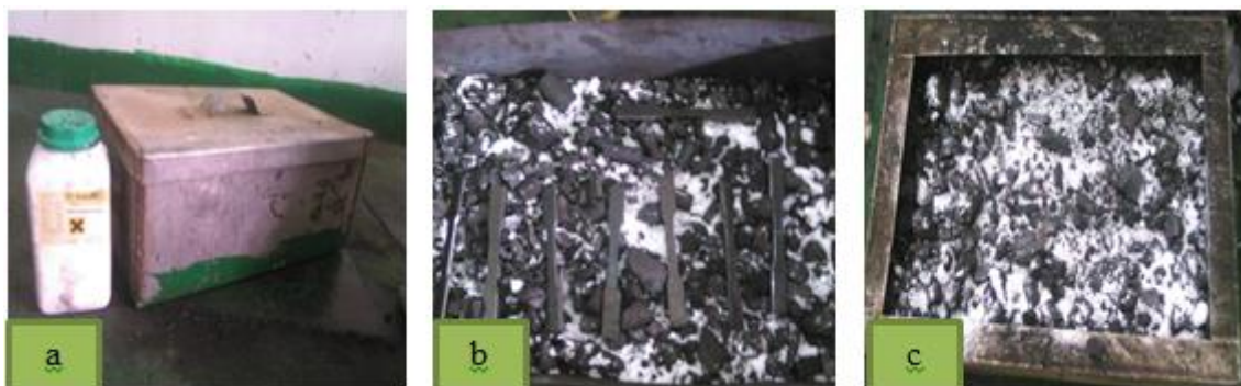
Figure 3-15 (a) NaCo 3 and Carburizing Box. (b) Samples Arrangement. (c) Samples Paced in the Box.
