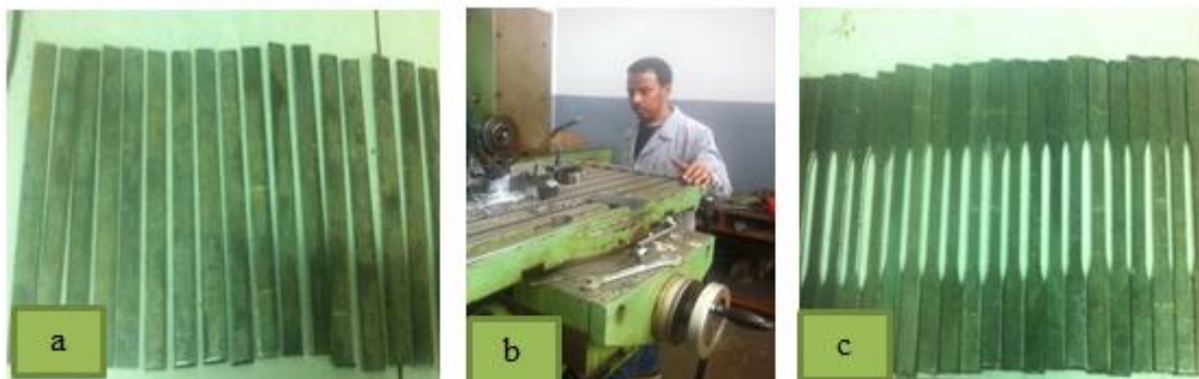
Figure 3-2 (a) Samples before machining. (b) Machining the samples (c). Samples after machining
