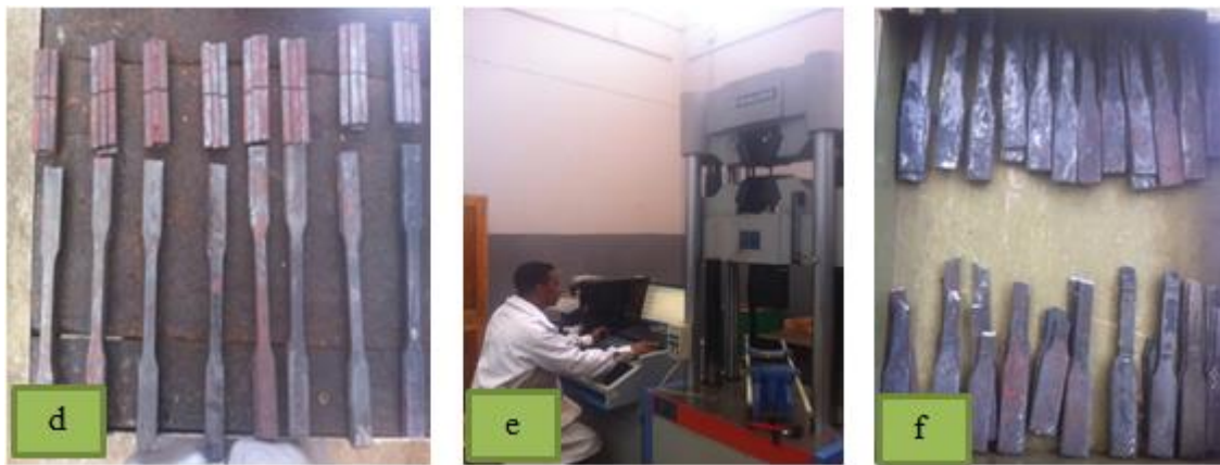
Figure 3-3 (a) Tempered samples before testing. (b) Testing samples on U.T.M. (c) Samples after testing.
