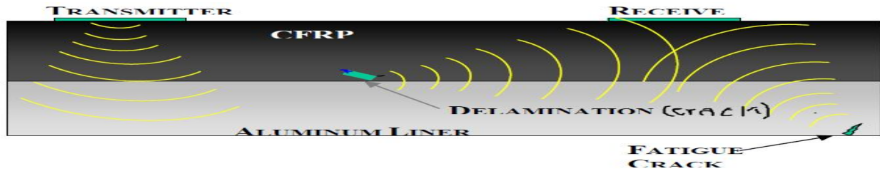
Fig 1 Acoustical Resonance System Schematic
