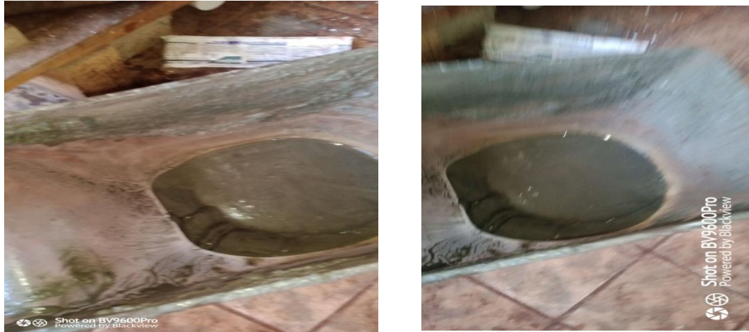
Figure 3 Iron concentrate deposited at the bottom of flotation cell after anionic reverse flotation carried out.
