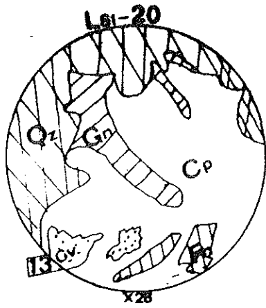
Fig.13 Galena (Gn) penetrating chalcopyrite (Cp) which contains fahlores (Fh). Cv (covellite), Qz (quartz).
