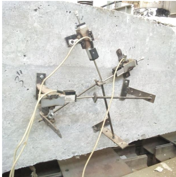
Figure 3-21 Surface Mounted Displacement Measuring Instruments
