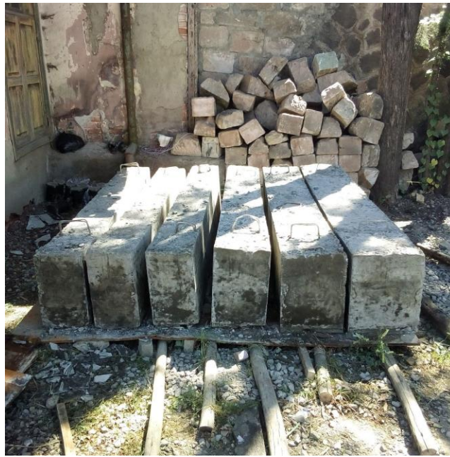
Figure 3-10 Beam specimens just after removal of formwork
