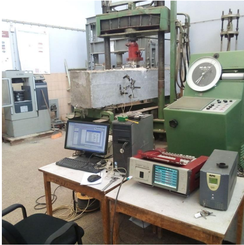
Figure 3-22 Geodatalogger Connected to a Computer Data Acquisition System
