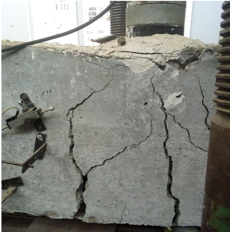
Figure 4-26 Final state Mid span cracking just before peak load SB-100
