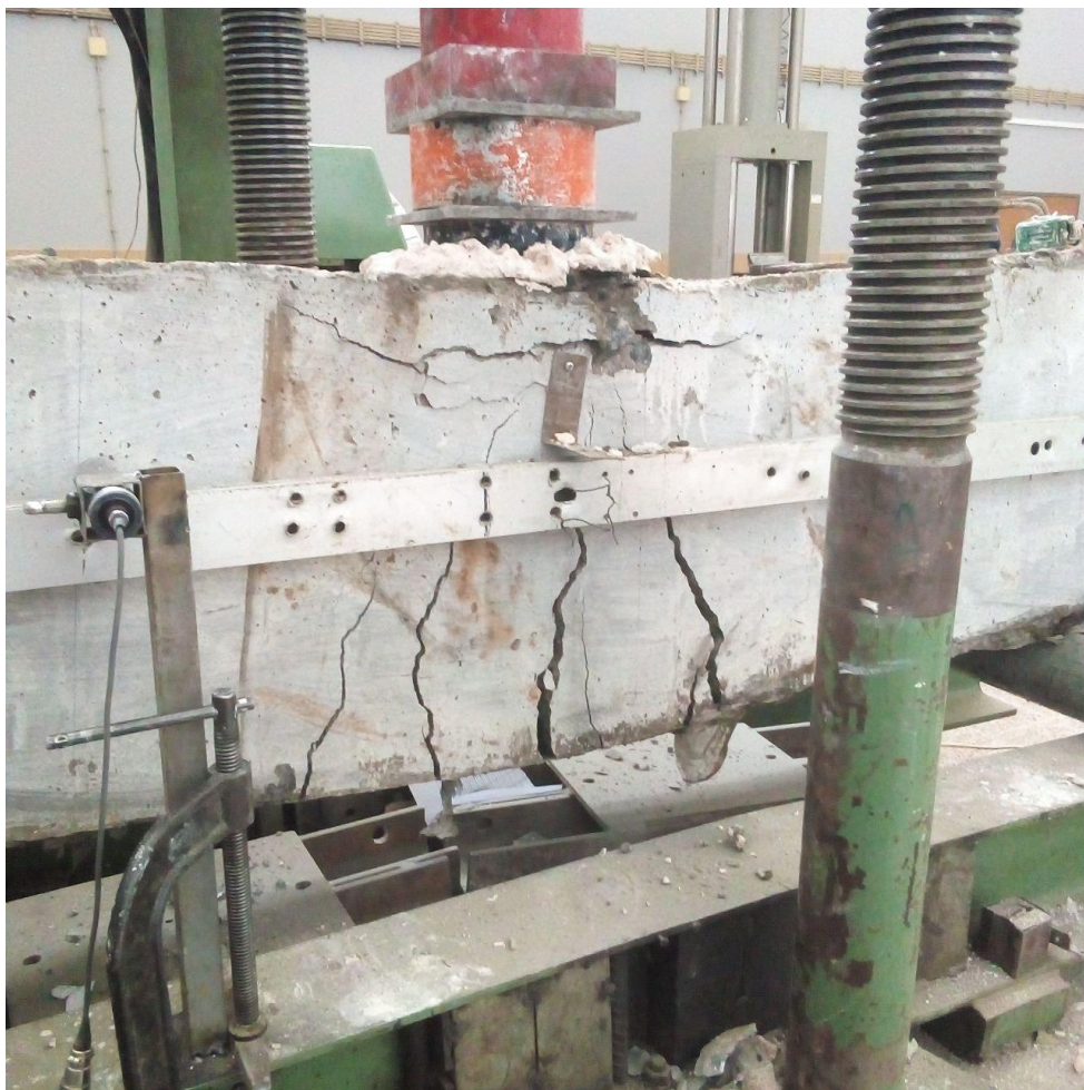
Figure 4-14 Final State of the Beam SA-75
