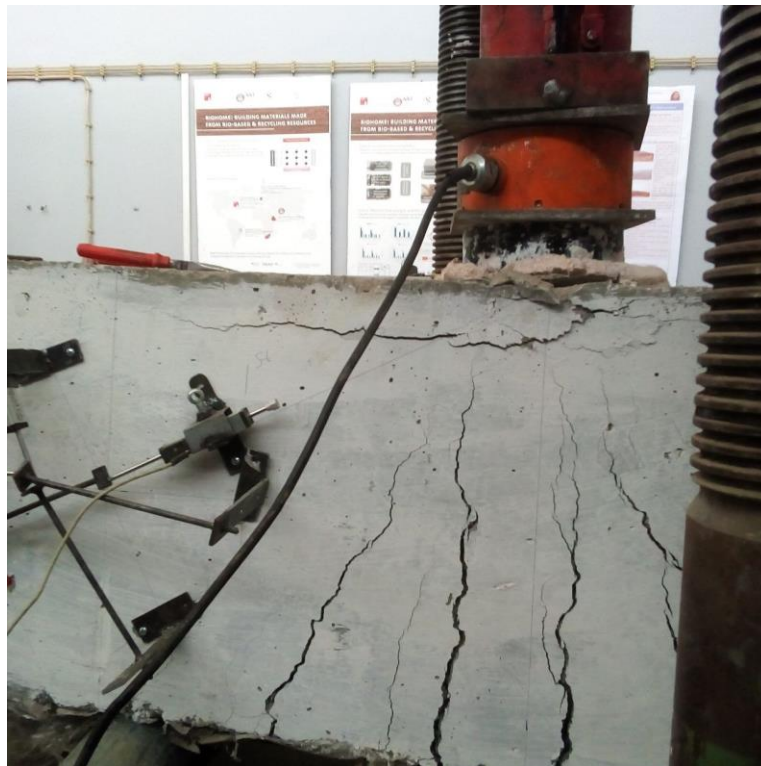
Figure 4-19 Final State of the Beam SB-50
