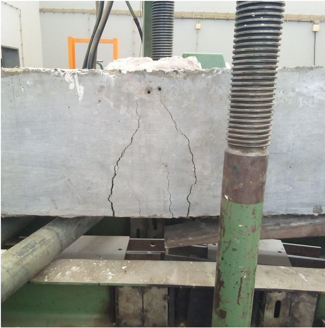
Figure 4-22 Final state Mid span cracking just after peak load SB-75
