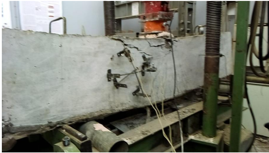
Figure 4-4 Side Cover Spalling Limited at the Top under peak load (SA-25)
