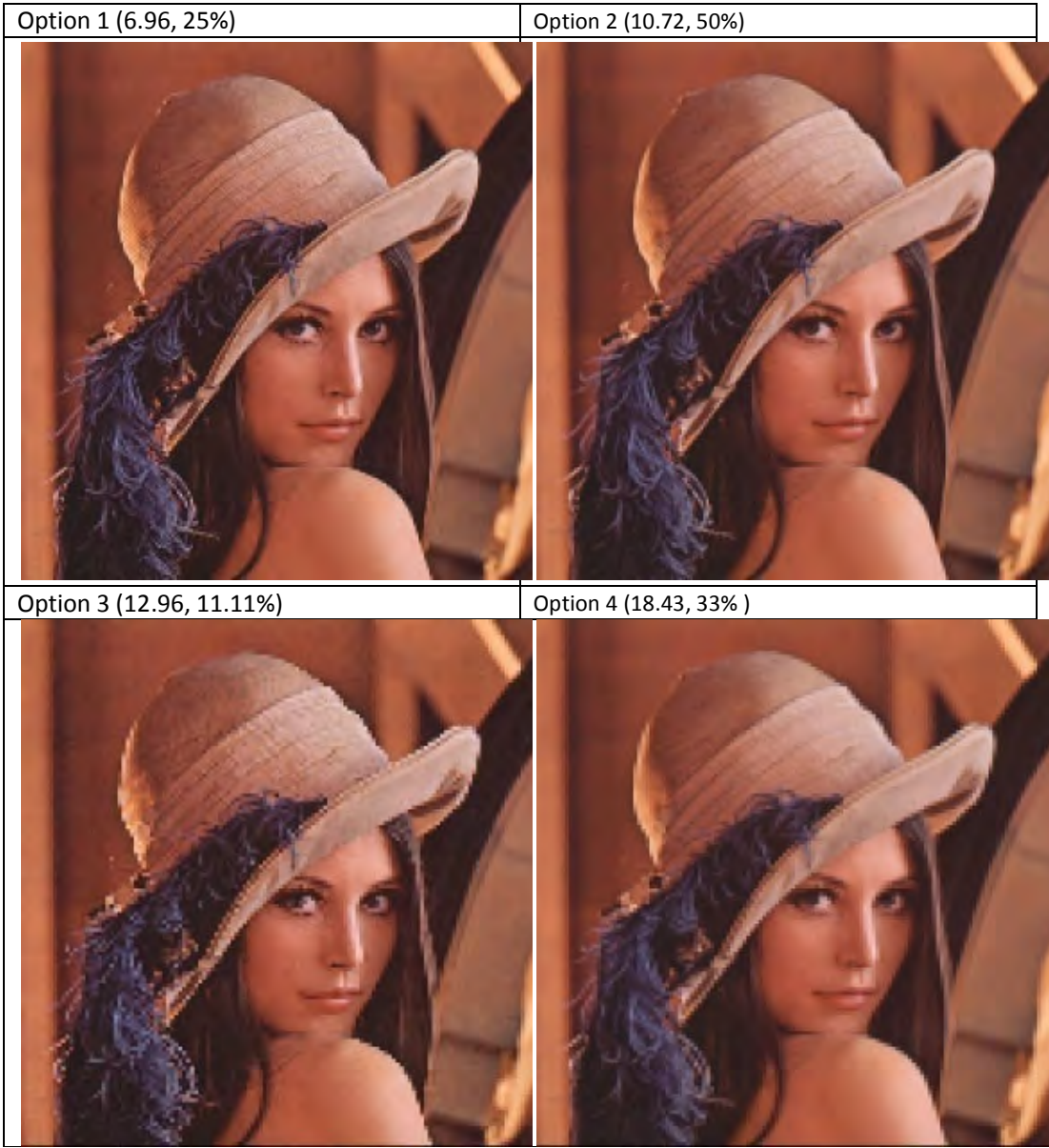
Figure 5-9b: Result of ALG3. The values in brackets are in the form (reconstruction error, compression ratio).
