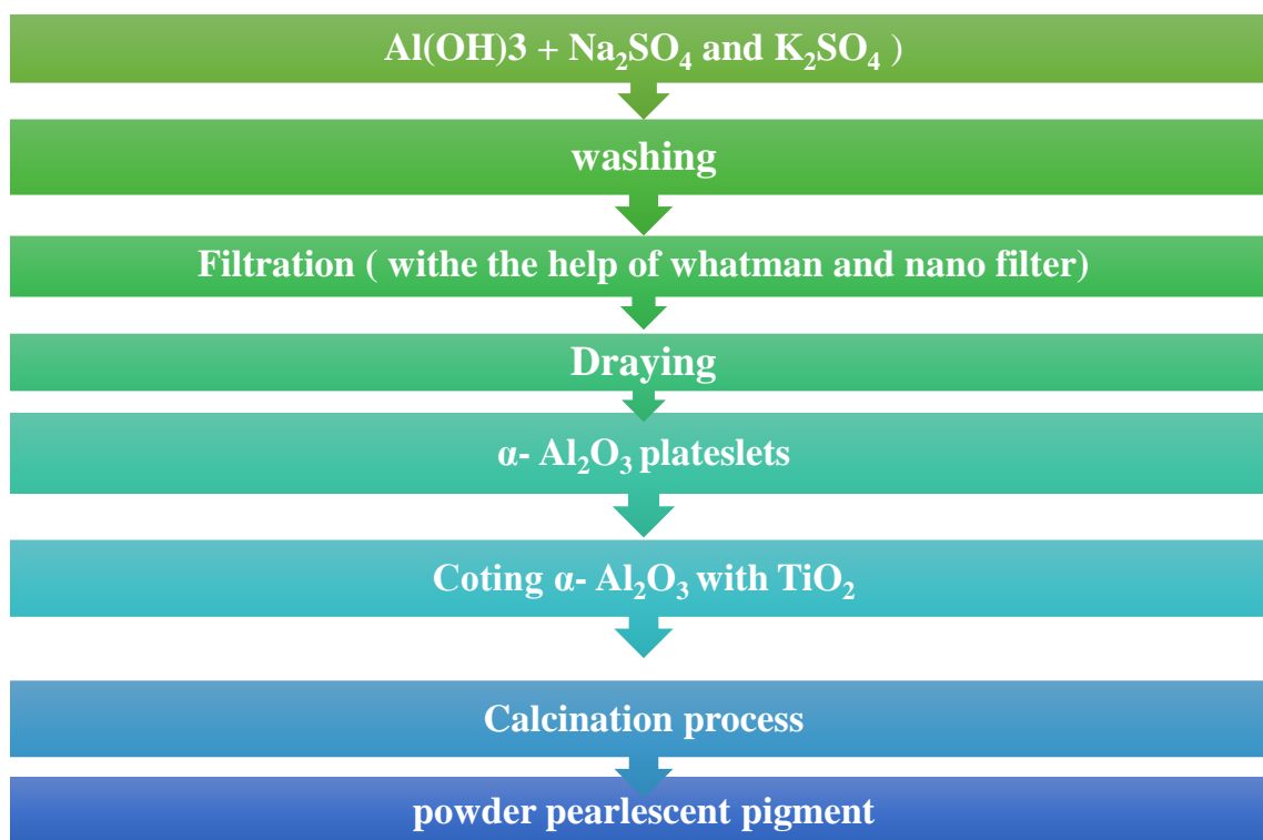
Figure 3.1: Process flow of \alpha\text{-Al}_2\text{O}_3 with \text{TiO}_2 pearlescent pigment
