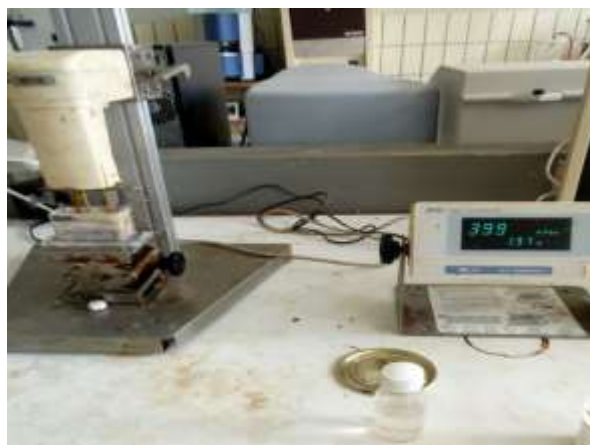
Figure 3. 4: Experimental setup for viscosity measurement
