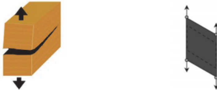
Figure 3.2 Mode I or opening mode [18]
