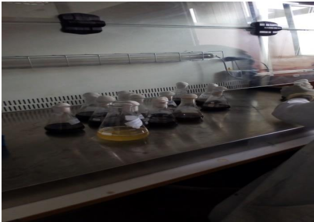
F9: v-cabinet hood instrument(laminar flow)
