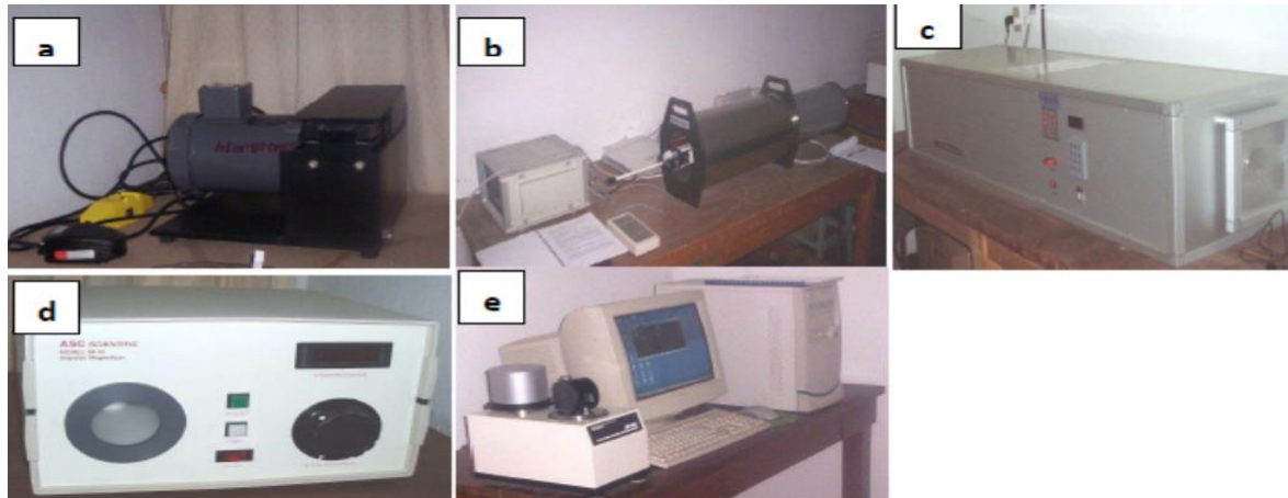
Fig.3.2. Instruments used in Laboratory (A) dual blade core slicer saw. It slices each sample from all sites into specimens. (B) LDA-3, alternating field demagnetizer. (C) MMTD 80 furnace thermal demagnetizer. (D) ASC-IM impulse magnetizer for acquisition of isothermal remnant magnetization. (E) JR6-A spinner magnetometer lined with a desktop computer to measure intensity of magnetization existed in: AAU in School of Earth Science.
