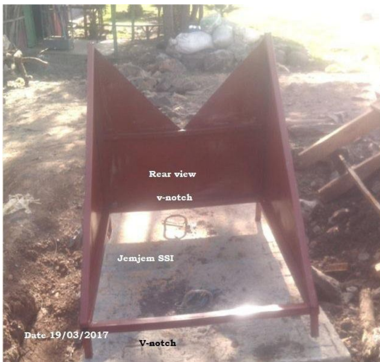
Figure B-5 90 degree v- notch weir prepared for canal discharge measurement
