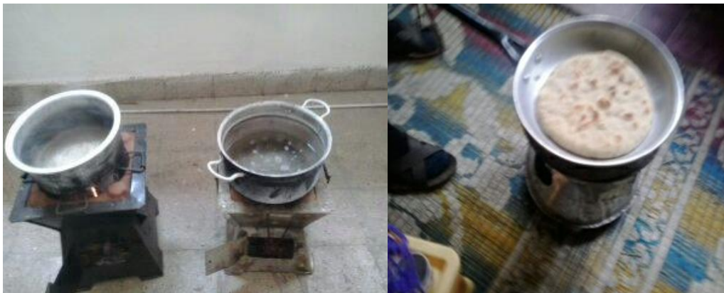
Figure3b Water boiling and cooking efficiency test on produced LC briquettes. Photo by SintayehuAbebe, 2015
