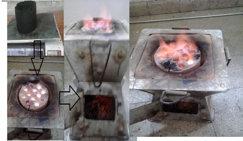
Figure3a weighing the produced LC briquettes and its burning qualities, giving a blue flame. Photo by SintayehuAbebe, 2015
