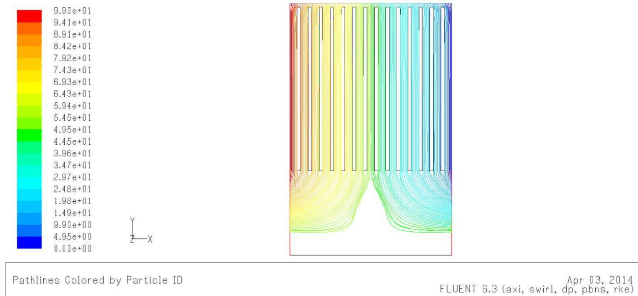
Figure 6-6: Fluid Pathlines for Two-Dimensional Numerical Model at Design Conditions
