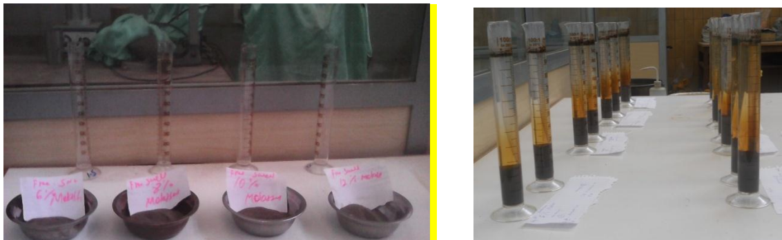
Figure 4. 7: (i) oven dried sample before test (ii) samples after final swelling
