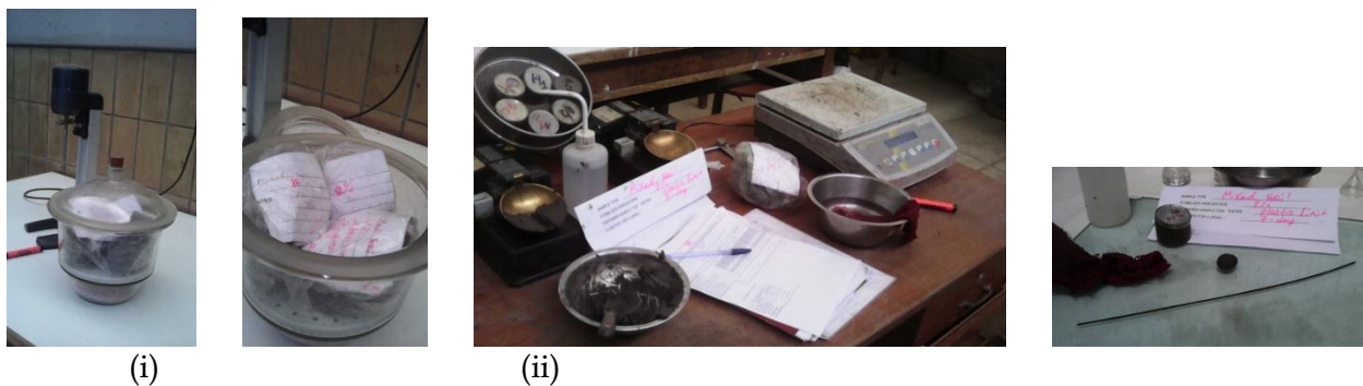
Figure 4. 4: sample curing (i), Atterberg limit testing
