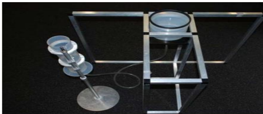
Figure 6: The custom-designed water displacement device used to measure breast volume.
