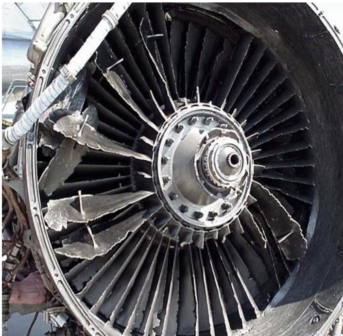
Figure 25 Jet engine damaged by wildlife strike
