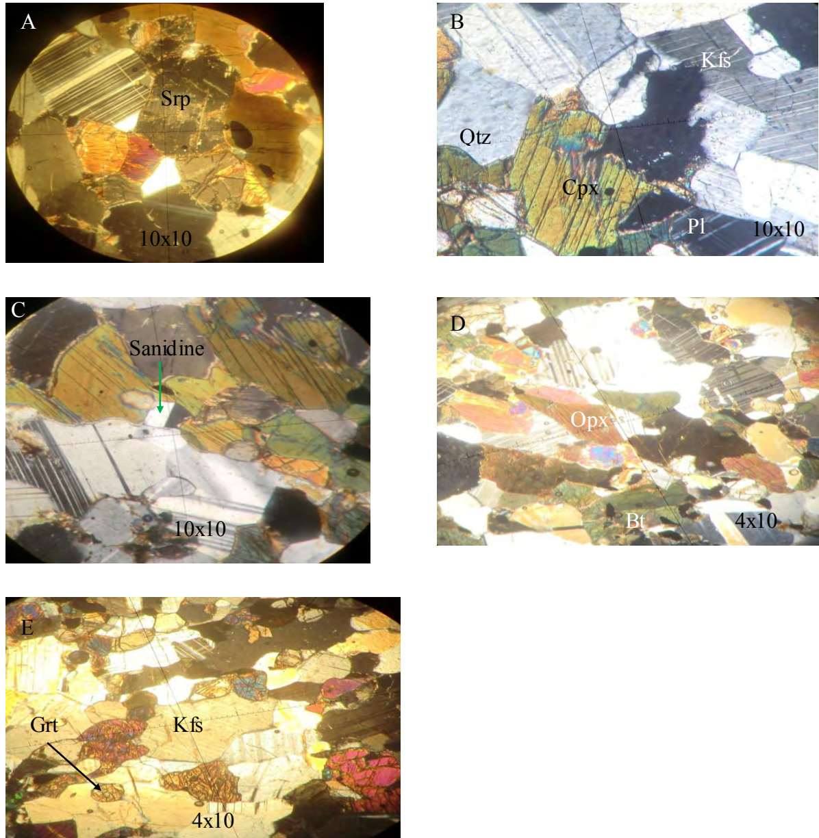
Figure 3.4 Photomicrographs mineral grains in charnockite rock. (A) Clinopyroxene shows serpentinization as well as being replaced by hornblende. (B) Broad grain of clinopyroxene surrounded by k- and plagioclase felds pars. (C) Small grain of sanidine (D) Broad twisted biotite with opaque inclusions. (E) Small euhedral garnet grain. All are seen under crossed polars.
