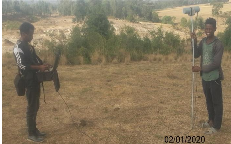
Figure 4. 3 Magnetic data acquisition using the proton precession magnetometer (GSM-19T).
