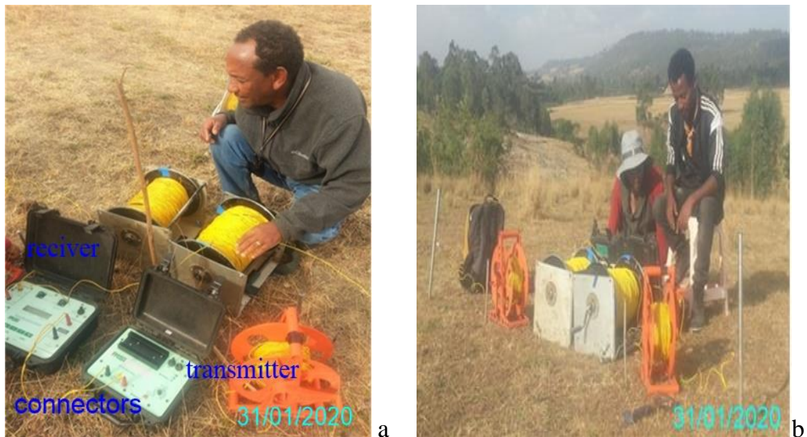
Figure 4. 2 Photo a) instrument field setup, and b) data acquisition scheme for the Vertical Electrical Sounding survey.
