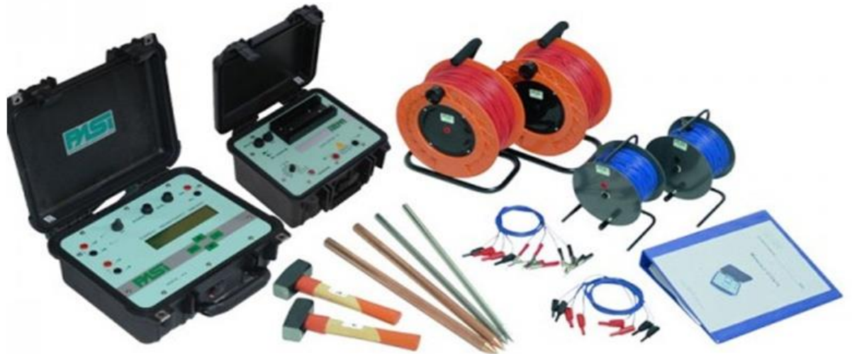
Figure 3. 1 Equipment layout for electrical resistivity survey (Image extracted from http://pasisrl.en.ecplaza.net )
