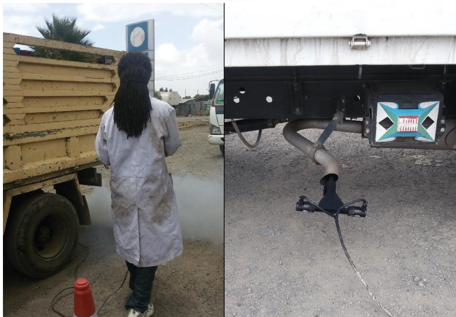
Figure 8: Pre clearing of the tailpipe before measurement (left) and opacity meter plugged on tailpipe (right)
