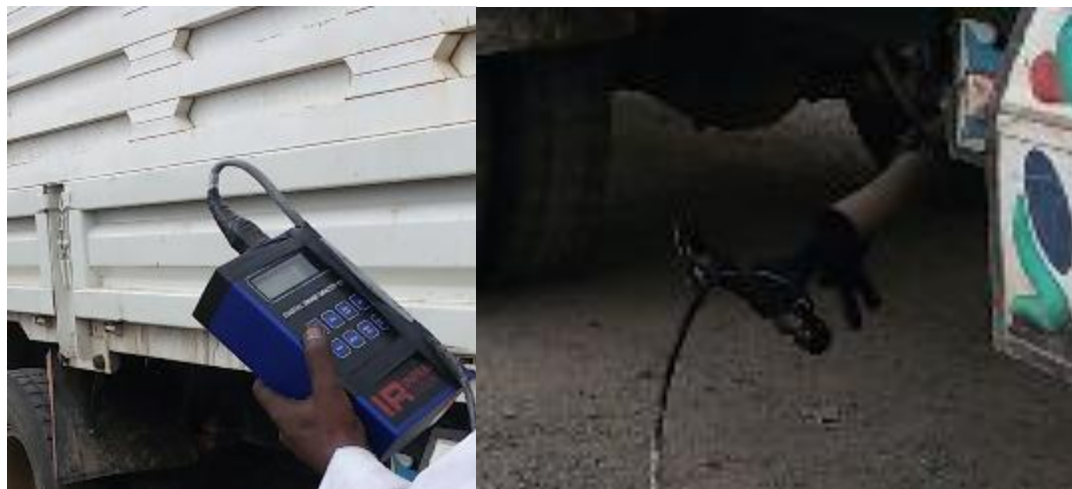
Figure 3: Opacity meter (Reading Monitor (Left) and tail pipe plug (Right))
