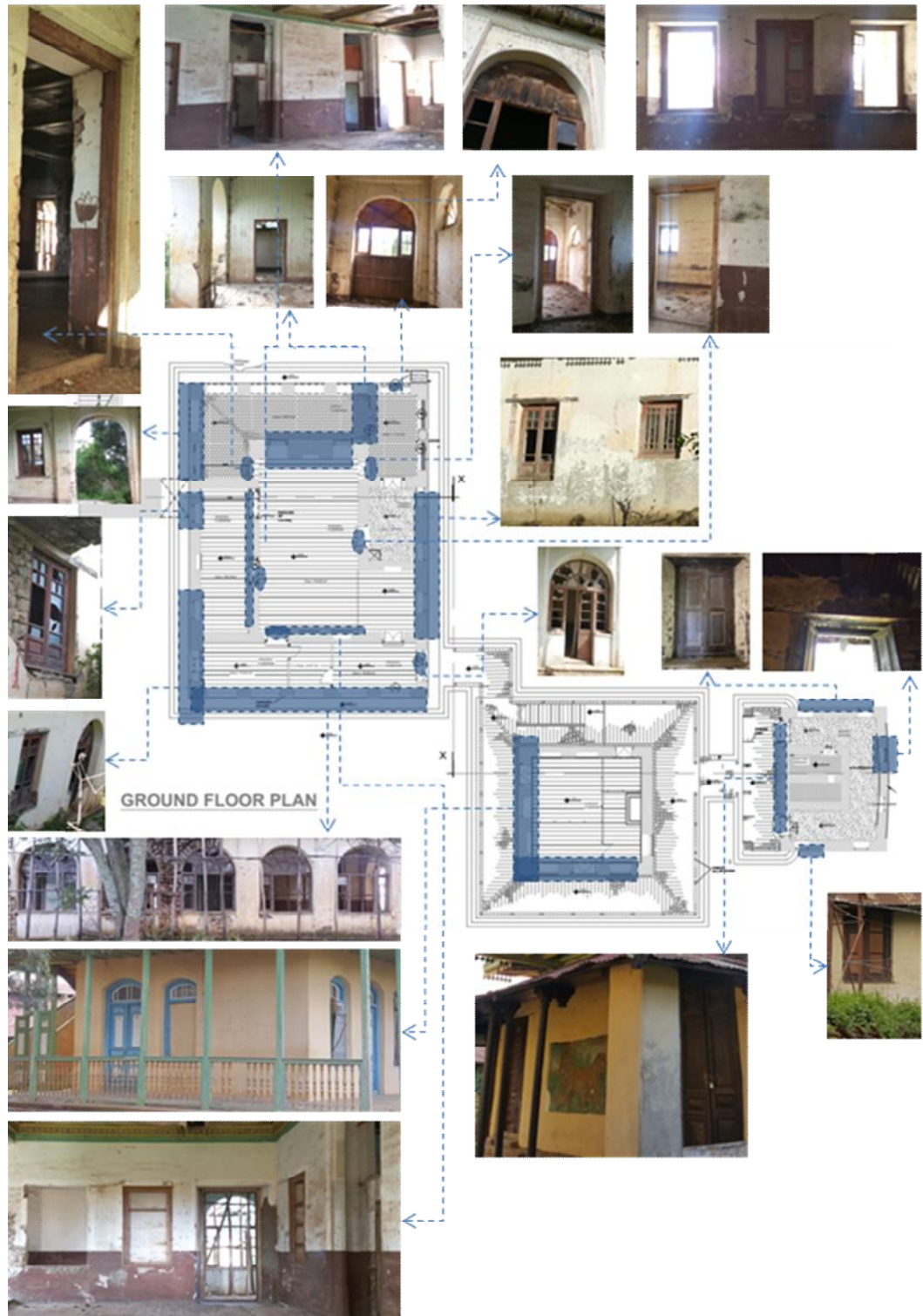
Figure 4.33 –doors & windows at ground floor level
