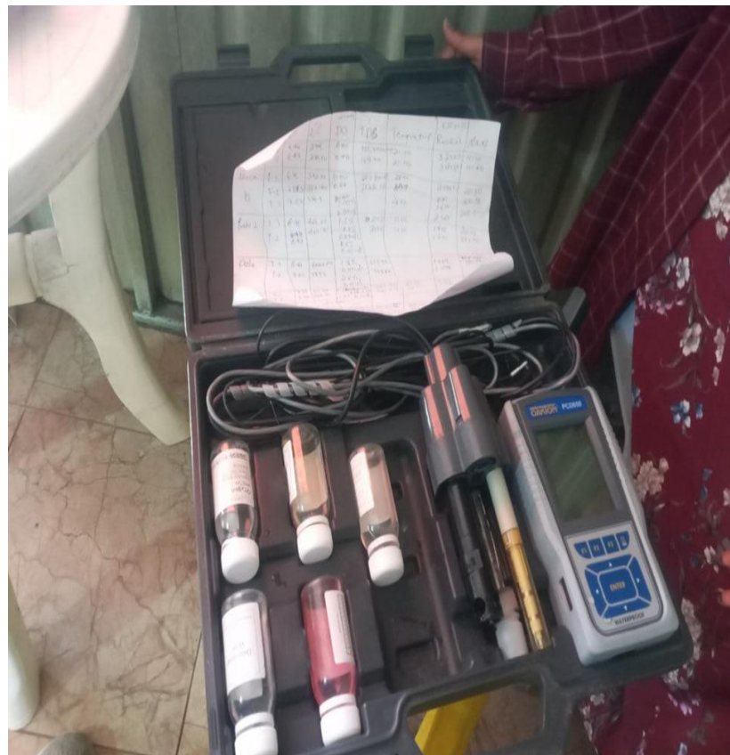
Picture 15 On situ measurement by OAKTON 600 series waterproof portable meter kit
