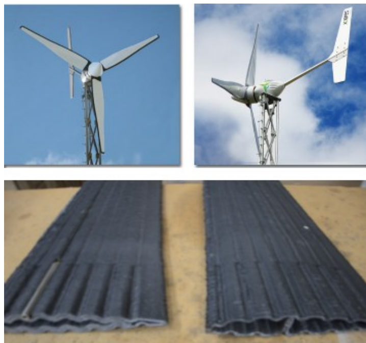
Figure 2.11: The adopted XZERES 442SR wind turbine (above) and the 3D printed blade sections (below) (B. K. Post et al., 2018)
