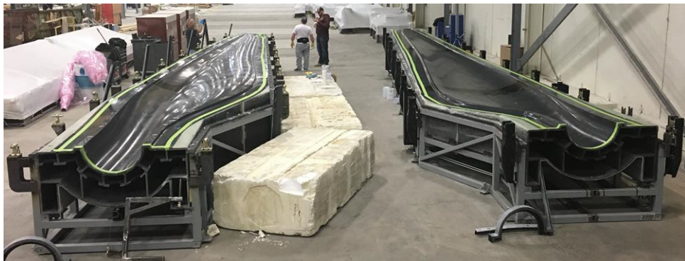
Figure 2.12: Final molds produced, upper and lower sections (B. Post et al., 2017)
