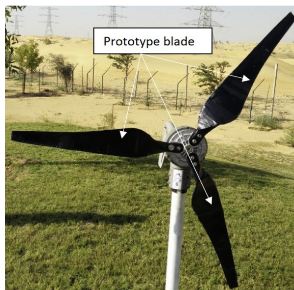
Figure 2.14: 3D printed blades on an AIR-X generator (Akour et al., 2018)
