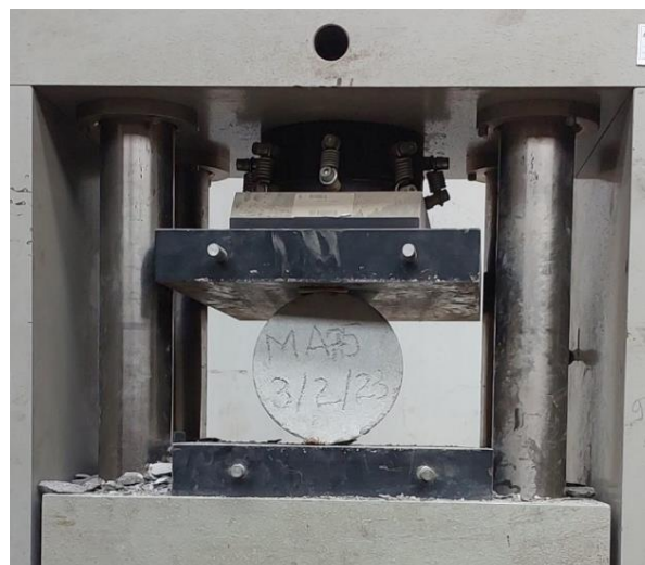
Figure 3.18 Splitting tensile strength test specimen setup
