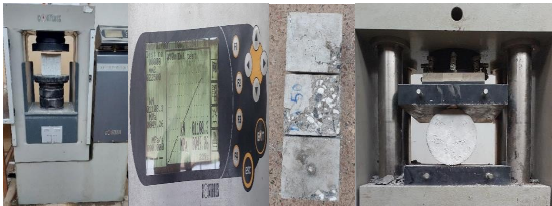
Compressive and splitting tensile strength test setup and failure of specimen
