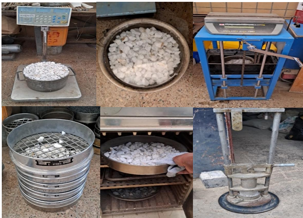
Laboratory test for marble aggregate (dry rodded unit weight, specific gravity and water absorption, gradation, oven drying, aggregate impact test)
