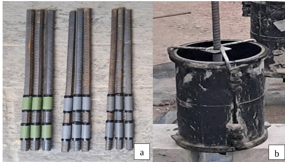
Figure 3.8 Specimen preparation a) diameter 12,14 and 16mm reinforcement bars with plastic conduit [right to left] b) cylindrical pullout mold with rebar at the center
