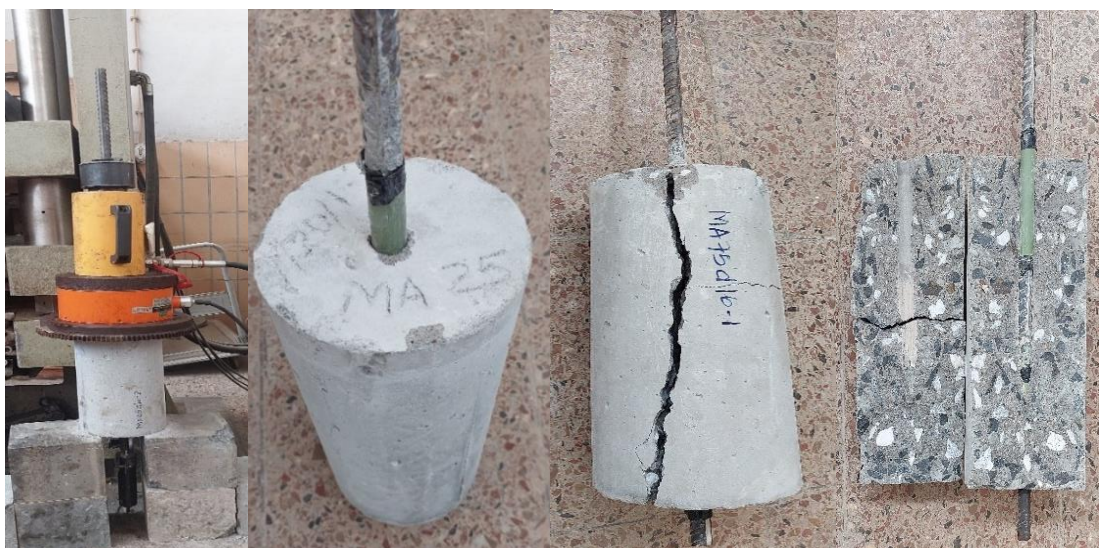
Pull-out bond strength test setup and failure of specimen
