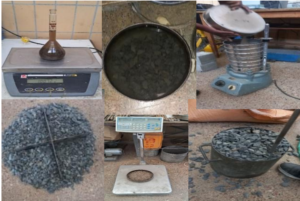
Laboratory test for fine and coarse aggregates (Sampling, specific gravity and water absorption, gradation, dry rodded unit weight, weighing)
