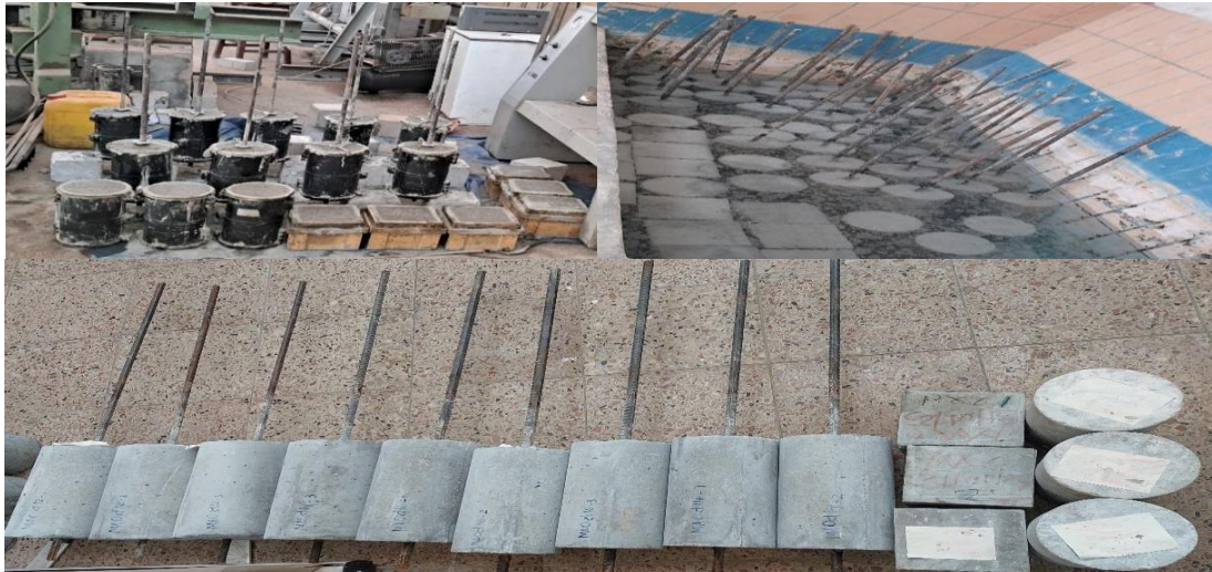
Concrete specimens casted, cured and ready for test
