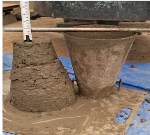
Figure 3.11 Measurement of slump for fresh concrete mix
