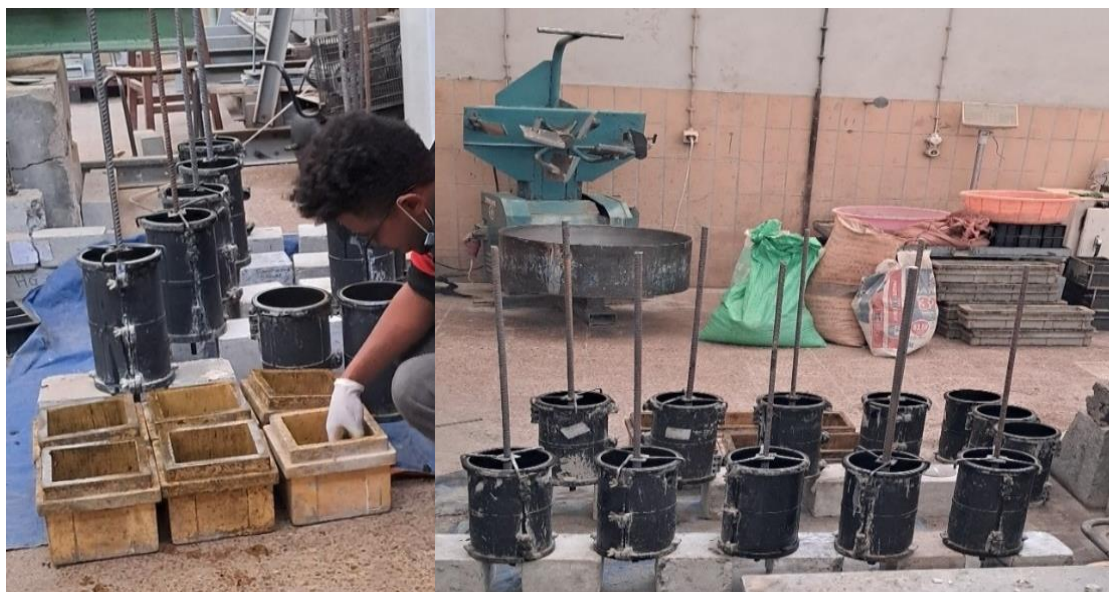
Figure 3.12 Oil coated molds ready for concrete casting
