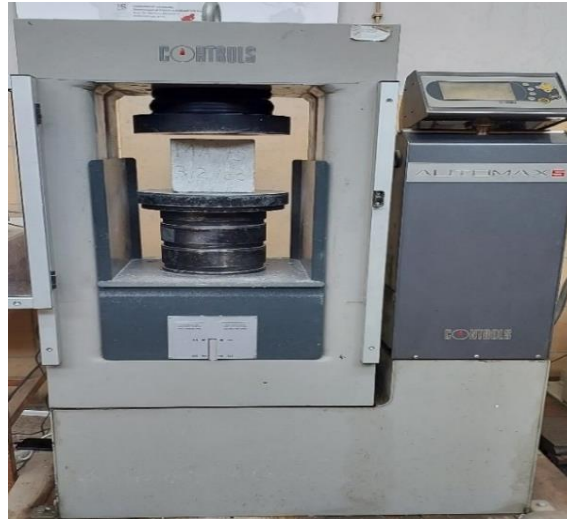
Figure 3.17 Compressive strength test specimen setup
