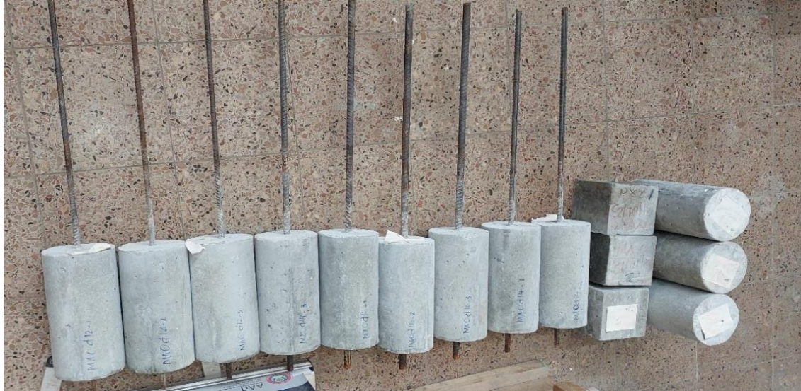
Figure 3.16 Concrete specimens ready for test
