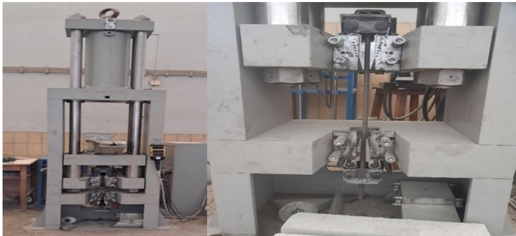
Figure 3.7 Tensile Strength test of reinforcement bars
