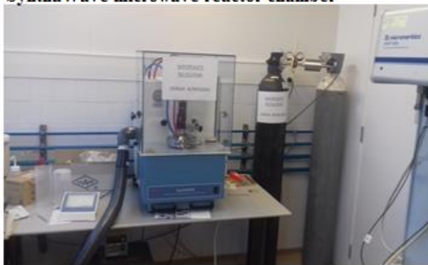
SynthaWave microwave reactor chamber
