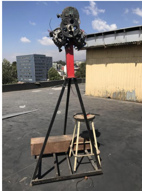
Figure 5.5.: Three small generators assembled with Frame
