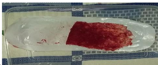
Figure 42: Absorbent capacity of the absorbent core of the proposed sanitary pad.
