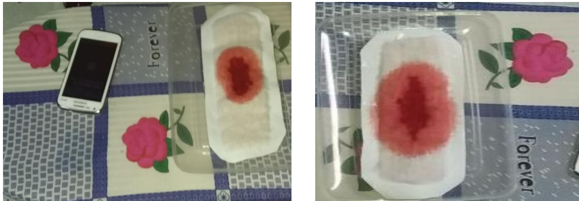
Figure 41: Images taken after 15ml and 30ml of colored fluid absorbed, respectively.
