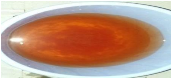
Figure 43: Image of a fully disintegrated absorbent core.
