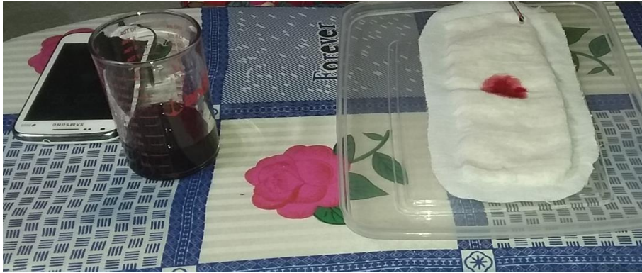
Figure 37:Image taken during liquid striking through test.
