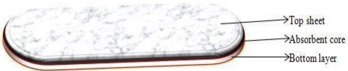
Figure 26: The composition of the proposed sanitary pad.
