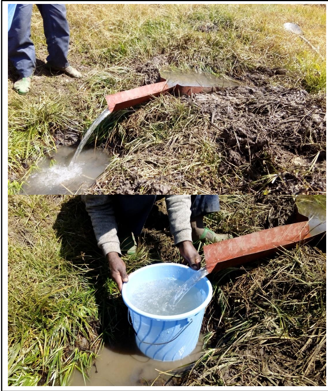
Figure 7. Measuring water flow at the outlets of the sites
