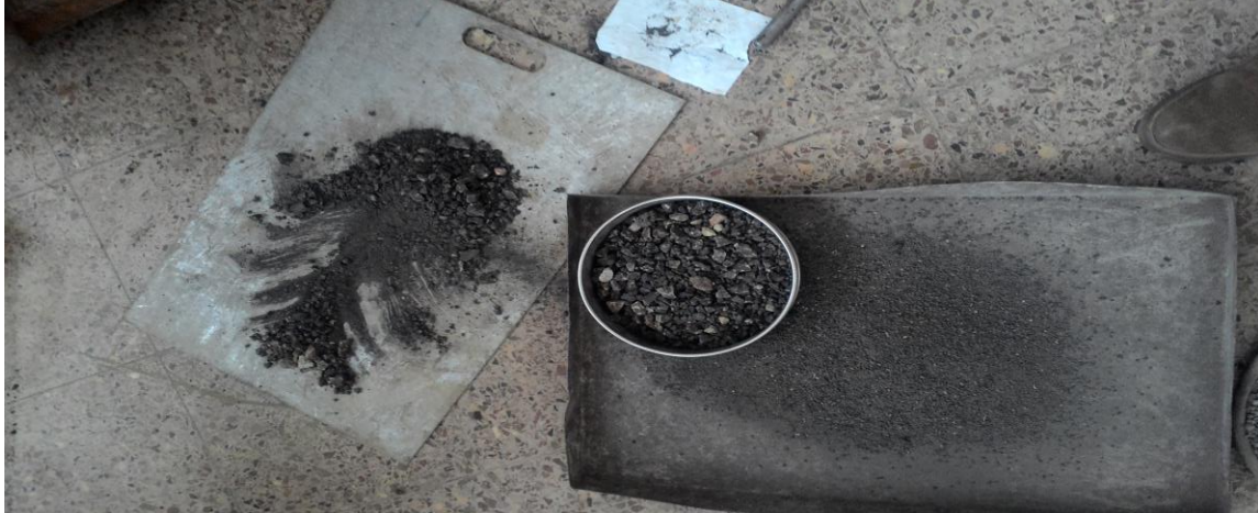
Fig. 3.33. Old track ballast during crushing and sieving
