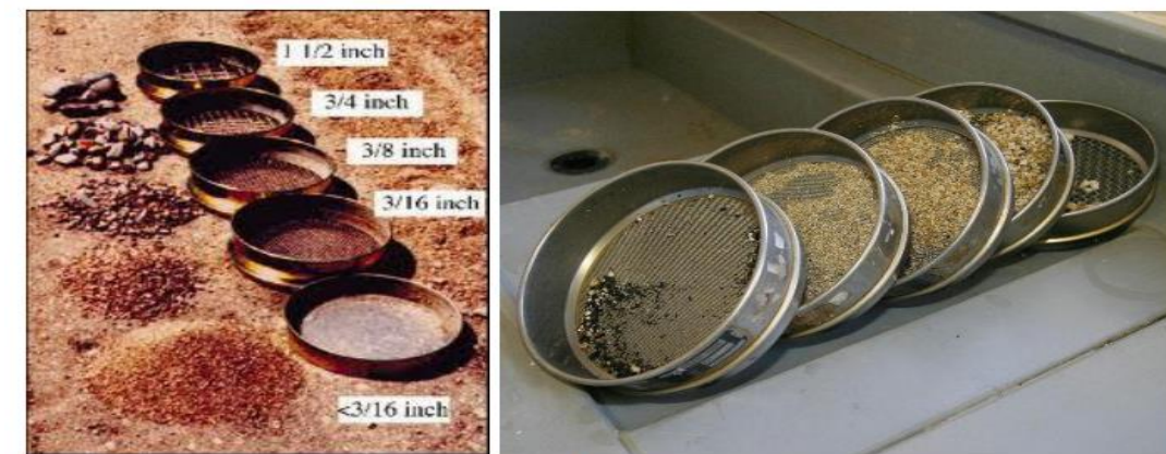
Fig. 2.8. Different sieve size (ASTM 2011)
