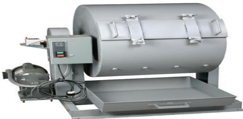
Fig. 2.9. LA abrasion testing instrument (ASTM, 2011)
