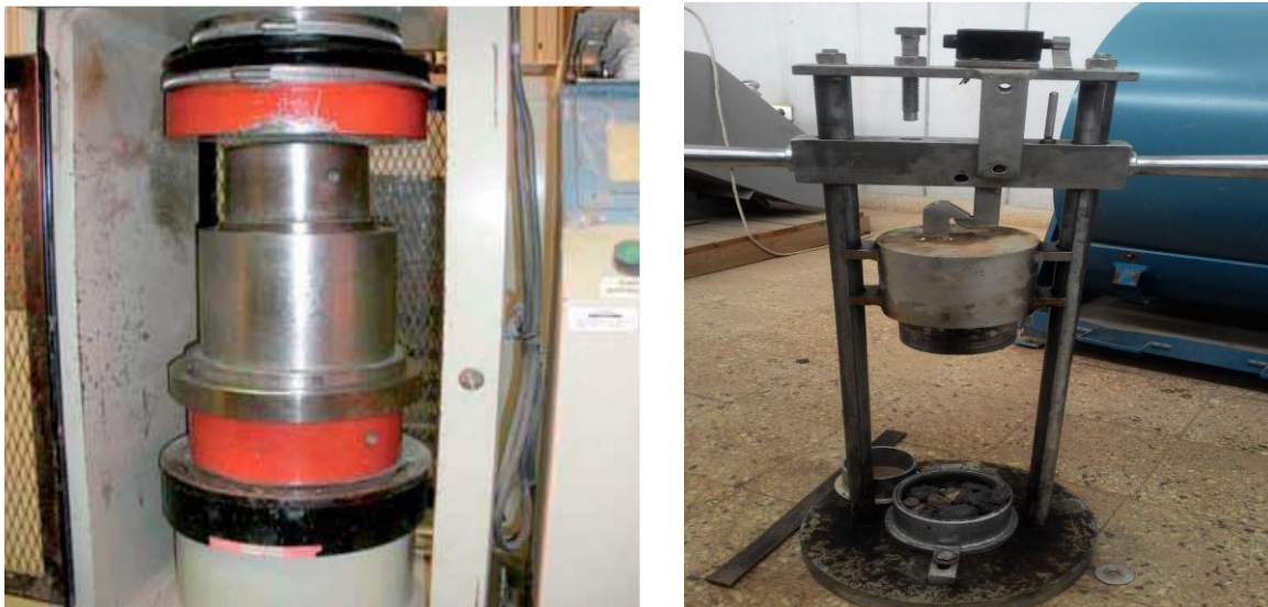
Fig. 3.32. AAiT crushing value and impact value testing machines for aggregate durability test
