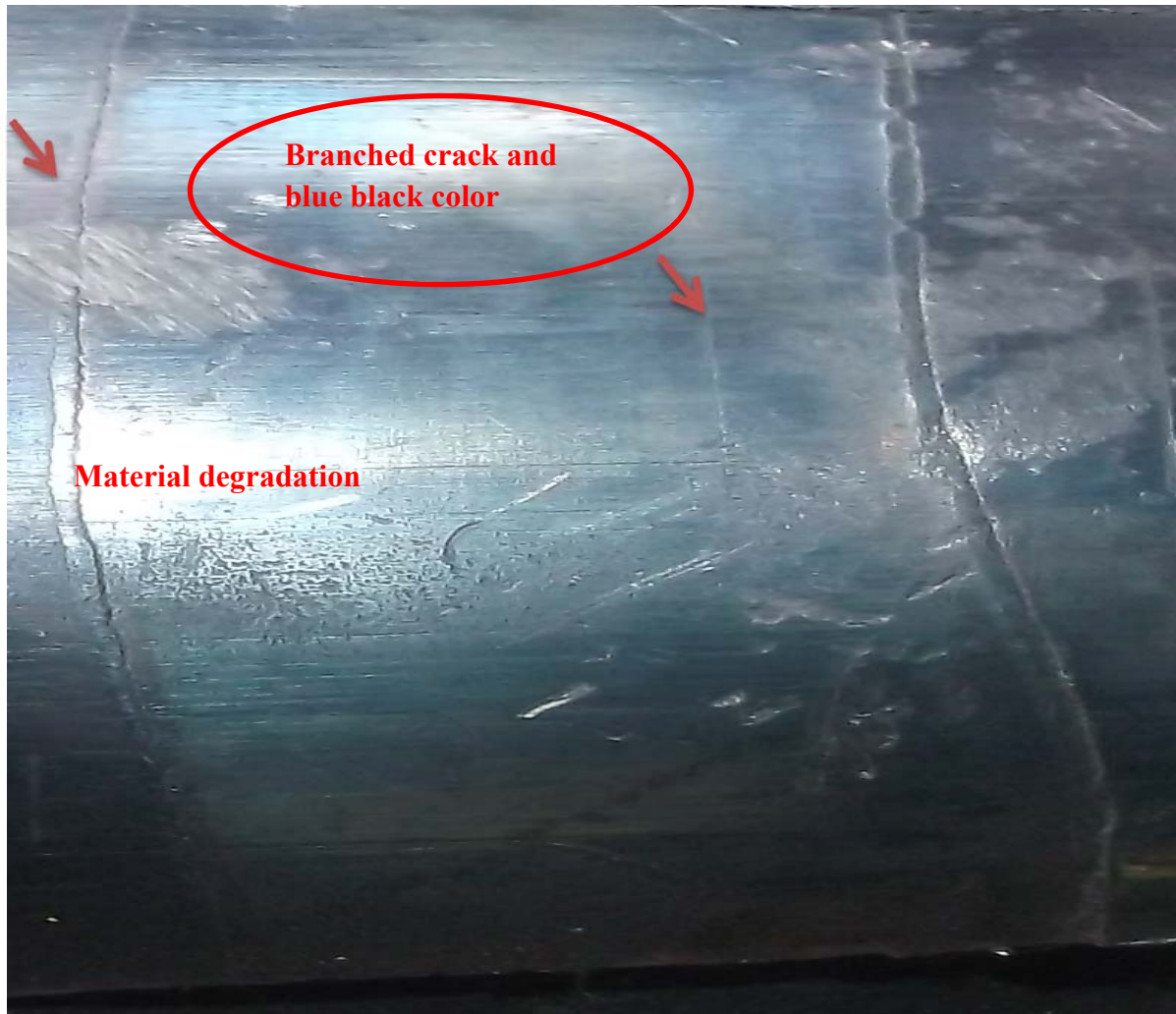
Figure 4-15: blue black color on the surface of site 3.2 and site 4 at a temperature of 34.43°C.
