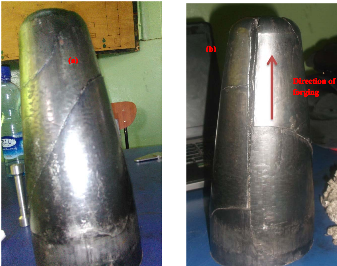
Figure 4-2: interlocked cracks at the back surface of the main cracks (a) back surface (b) main crack surface
