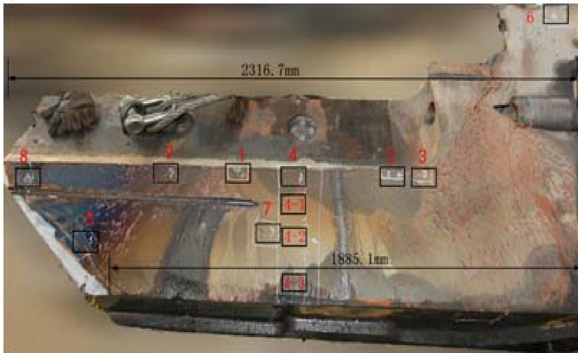
Figure 4-13: The whole fracture appearance and specimen's number. (source: Engineering Failure Analysis: Failure Analysis of large press die holder named by Hongxun Wanga, Peng Jiang, Weifang Zhang, Yaozhong Zhang, Tong Song; 6 April 2015 china )
