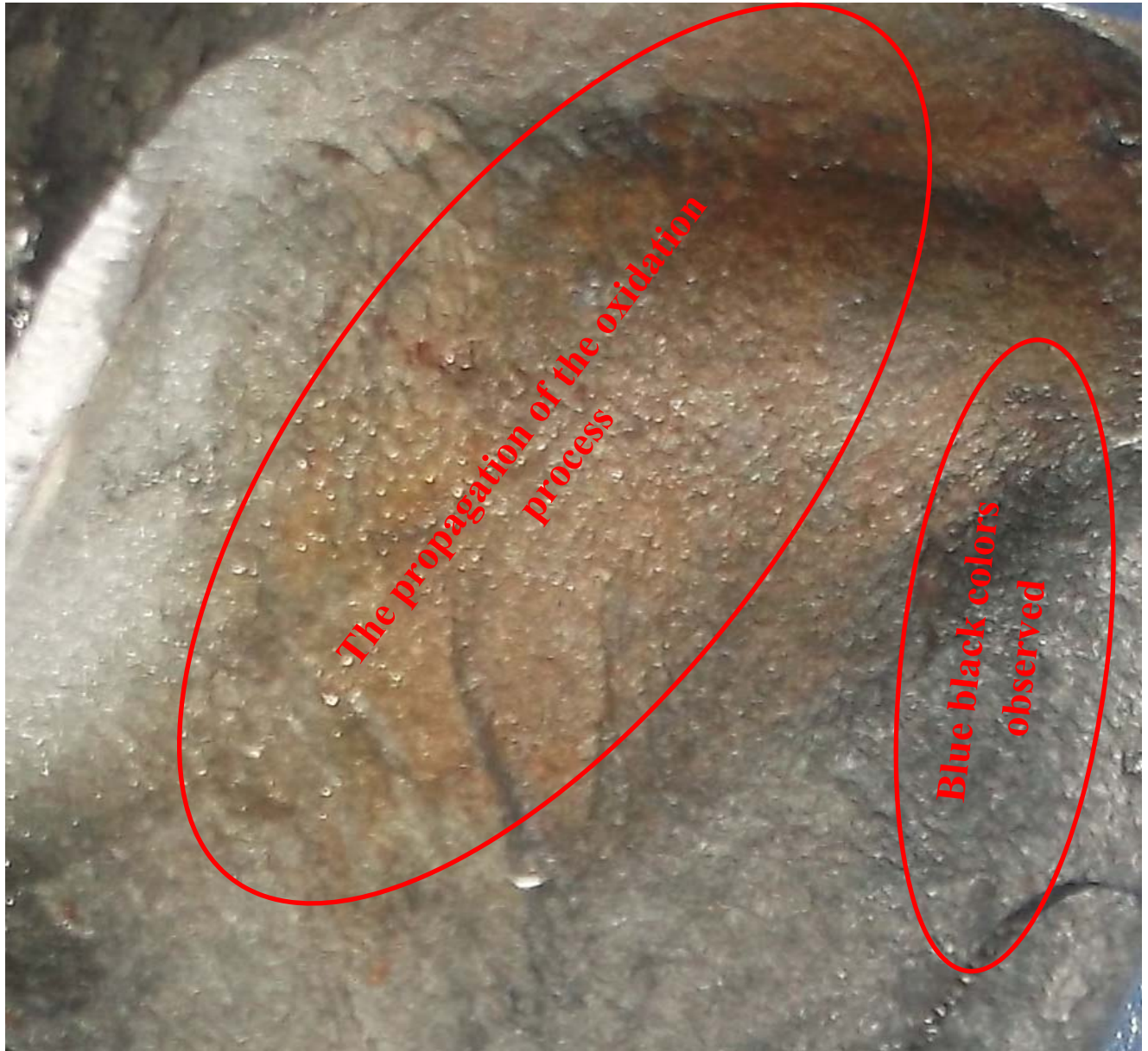
Figure 4-19: observation of oxidation layer on the puncher surfaces that is heated at a temperature of 180 0 C
