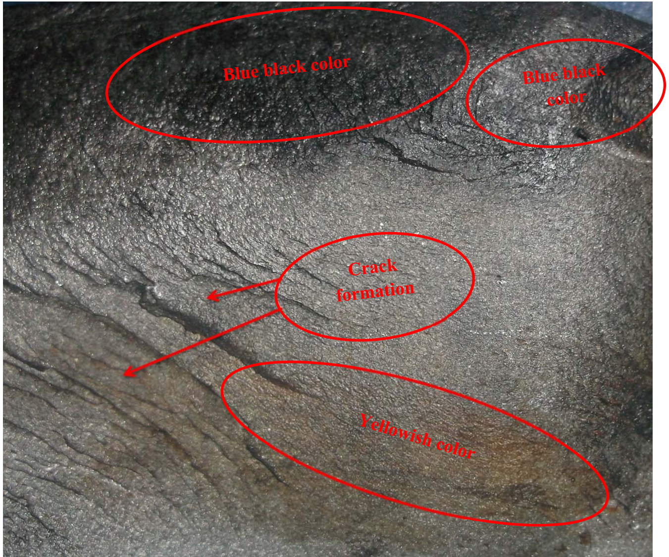
Figure 4-16: the yellowish color observed at site 4 of the puncher at a temperature of 34.43°C
