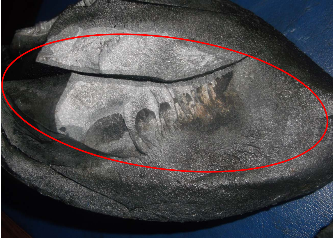
Figure 4-12: observation of yellow -blue- black oxidation layer at ambient temperature
