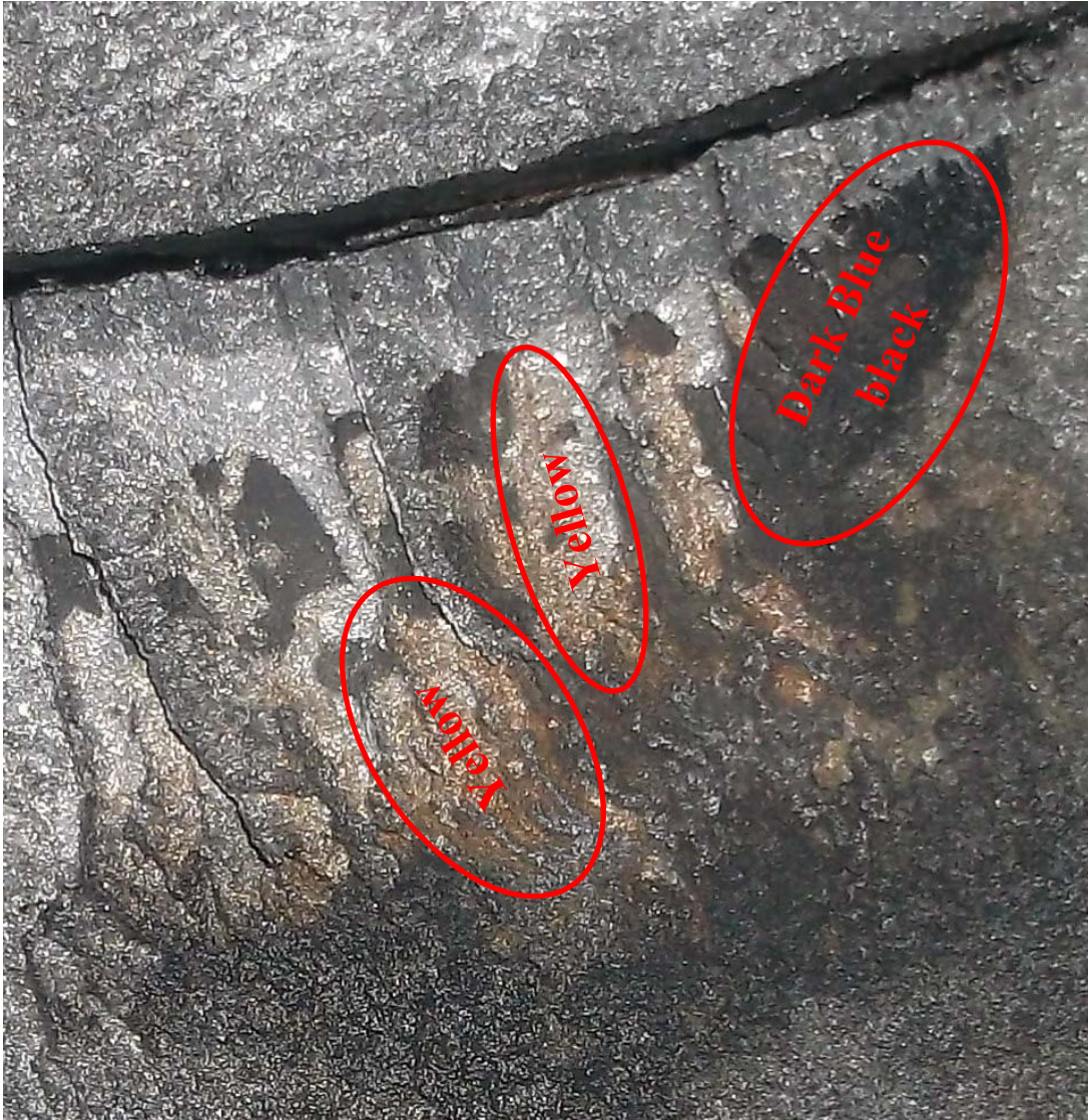
Figure 4-18: observation of oxidation layer on the puncher surfaces that is heated at a temperature of 140°C
