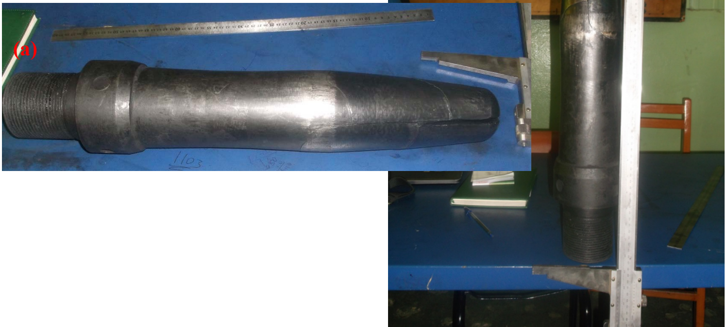
Figure 3-3: puncher profile manufactured in Homicho (a) in its horizontal position (b) in its vertical but opposite direction
