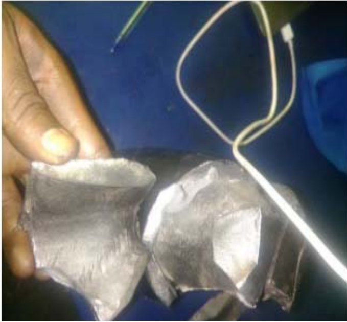
Figure 4-29: layer formation of the broken pieces
