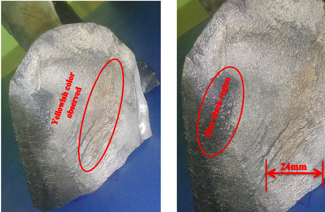
Figure 4-6: The broken image of piece 2
