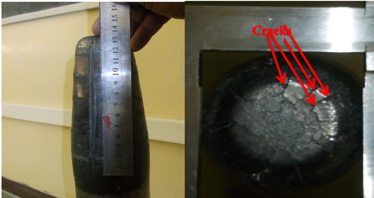
Figure 3-4: Crack extension length a) crack on the surface profile b) crack on the tip profile
