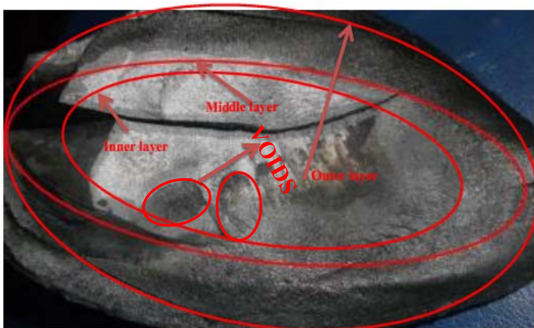
Figure 4-27: different surface cracking zone observed by other researchers (source: Engineering Failure Analysis: Failure Analysis of large press die holder named by Hongxun Wang, Peng Jiang, Weifang Zhang, Yaozhong Zhang, Tong Song; 6 April 2015 china) [25] [9] [26]
