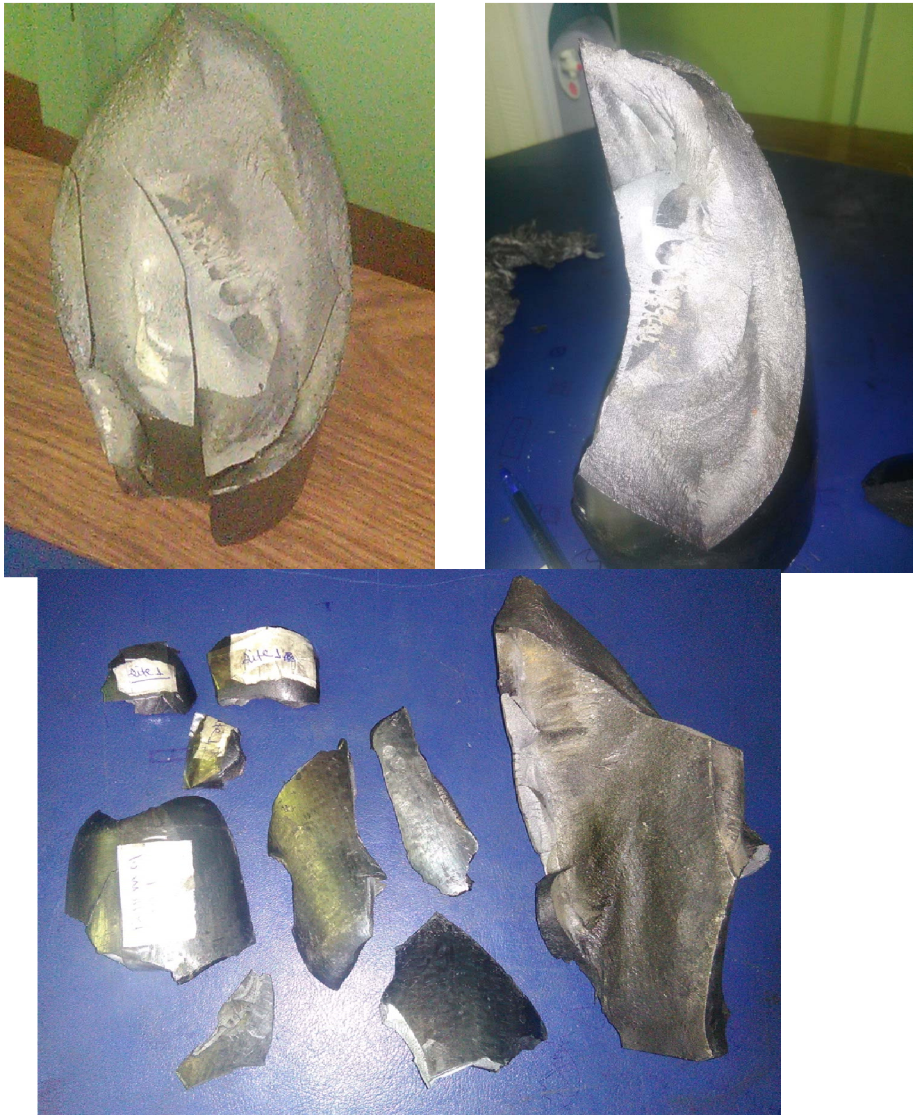
Figure 4-7: The subdivisions of piece 3 in to ten sub divisions (one of the ten is on machining for tensile testing samples)
