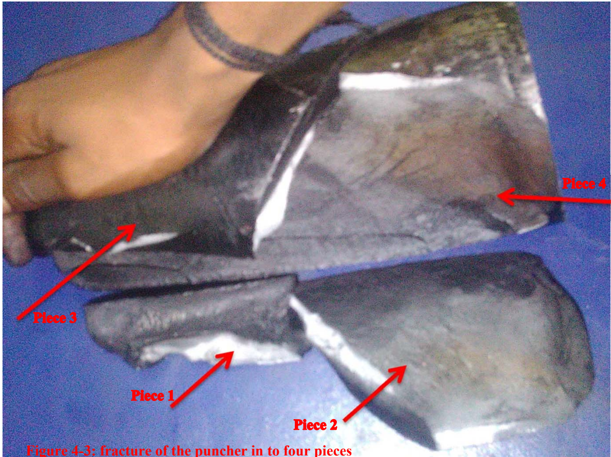
Figure 4-3: fracture of the puncher in to four pieces
