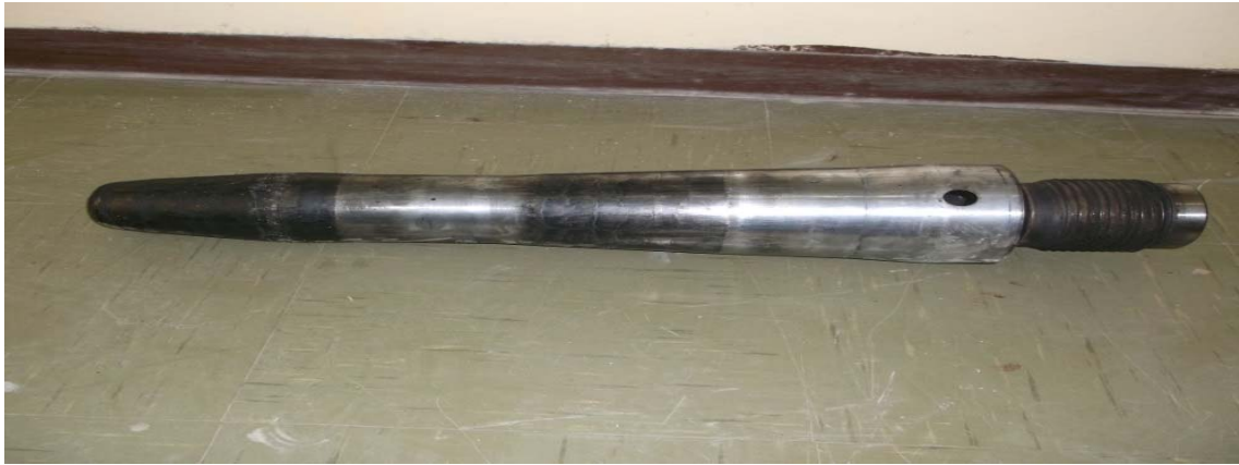
Figure 3-2: Korean drawing punch in its horizontal position
