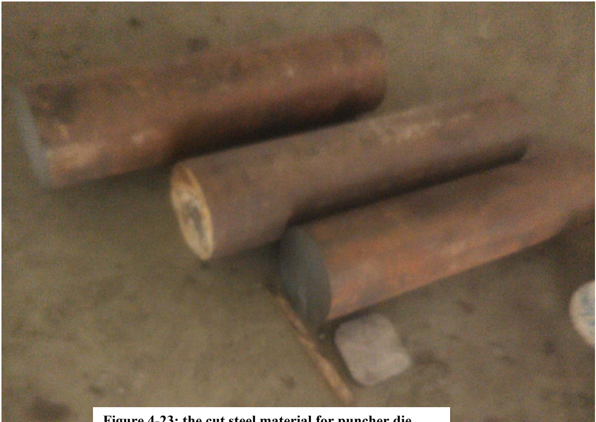
Figure 4-23: the cut steel material for puncher die
