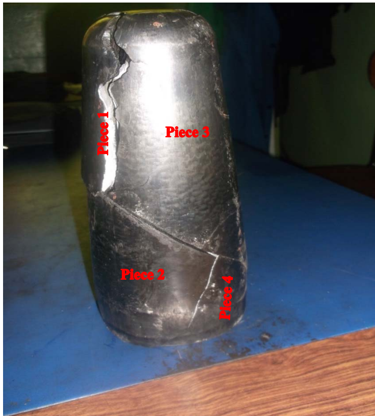
Figure 4-10: the assembly of the broken pieces
