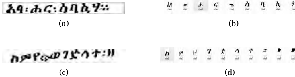
Figure 5.7: Output of errored segmentation: (a) input image (b) segmenting two characters as one (c) input image (d) segmenting one character by splitting in to two characters
