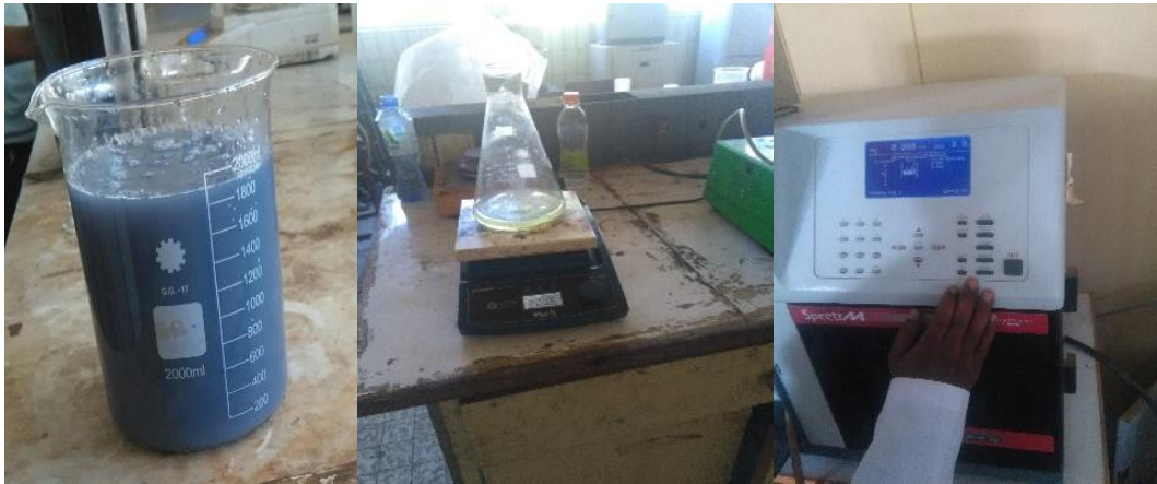
Figure 3. 2:Cr analysis (A) waste water sample, (B) Digestion and (C) Cr analysis using AAS
