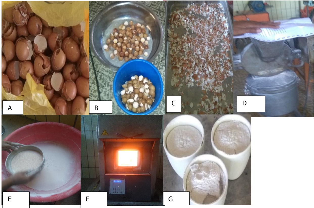
(A) Collection of eggshell, (B) Removing impurities by distill water, (C) drying, (D) grinding (E) Sieving, (F) calcination process and (G) Calcinated eggshell powder
