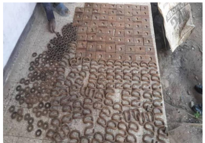
Figure 4.1: Fish plates, bolts, nuts and rail clips
