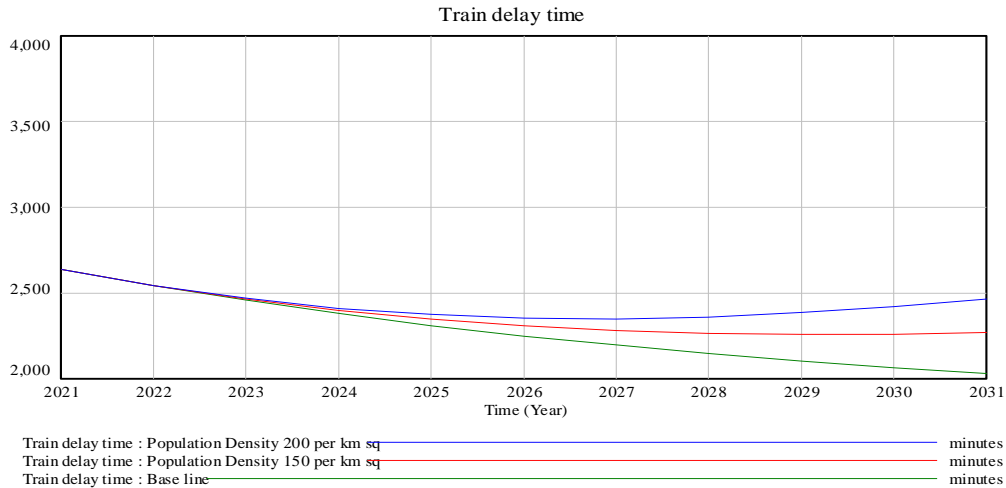
Figure 6.10: Simulation result of Train delay time by varying population density with 150 /km 2 and 200 /km 2
