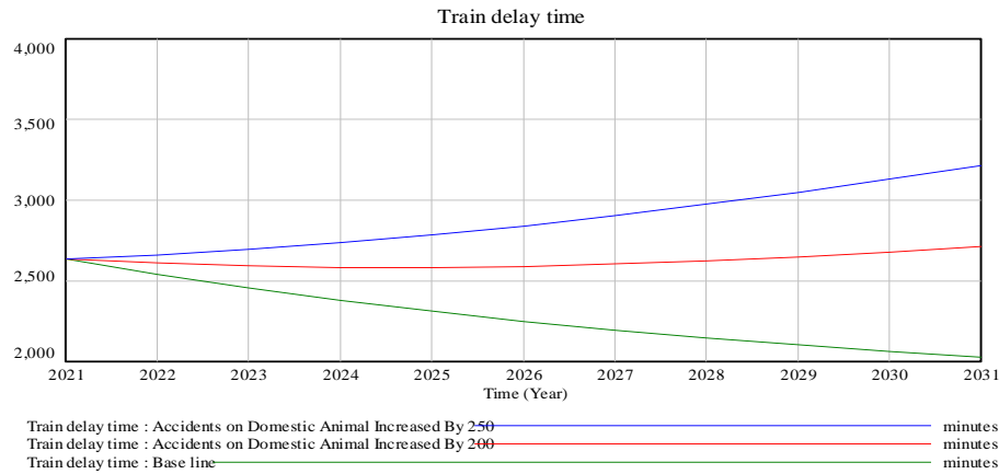
Figure 6.6: Simulation result of Train delay time by increasing Accidents on Domestic Animals with 200 and 250
