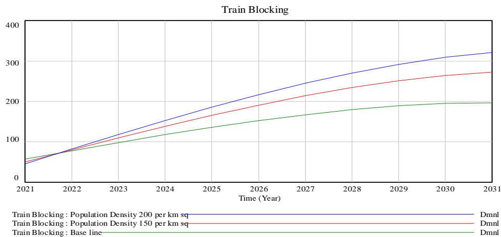
Figure 6.11: Simulation result of Train Blocking by varying population density with 150 /km 2 and 200 /km 2
