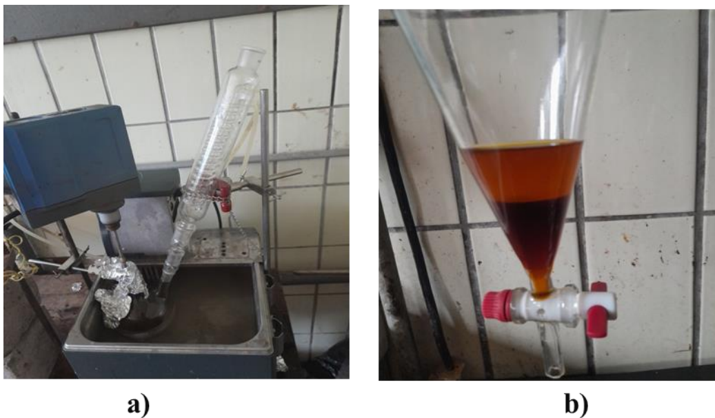
Figure 3.4 (a) experimental setup for transesterification reaction, (b) produced biodiesel
