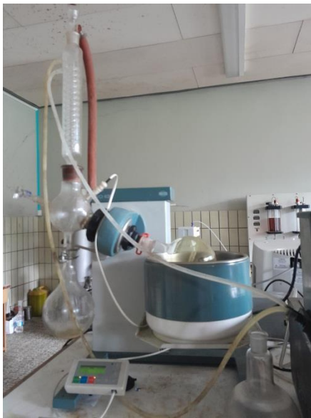
separation of oil from n-hexane(Vibro evaporator)
