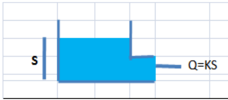
Figure 4.4: A realization of a single linear reservoir is a box with a porous outlet, thus obtaining Equation (4.1) from Darcy's law.
