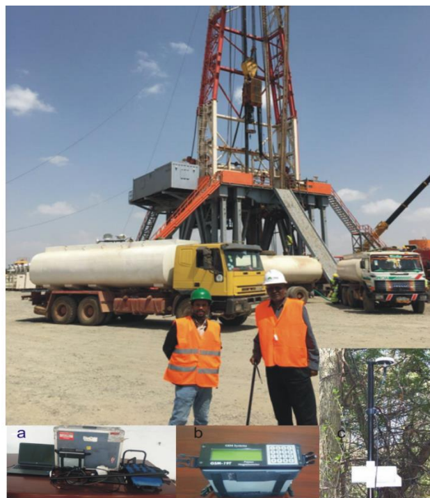
Figure 4. 2 instrumentation and data acquisition of magnetic survey: packing box(a), reading and recording instrument(b), GPS antenna (top white circle) and sensor (bottom white) (c).
