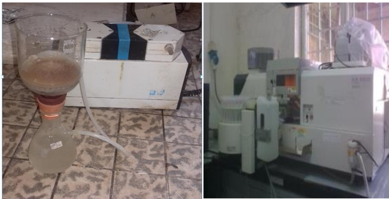
Figure D5: a) filtration of salt solution b) Flame atomic absorption spectrometer
