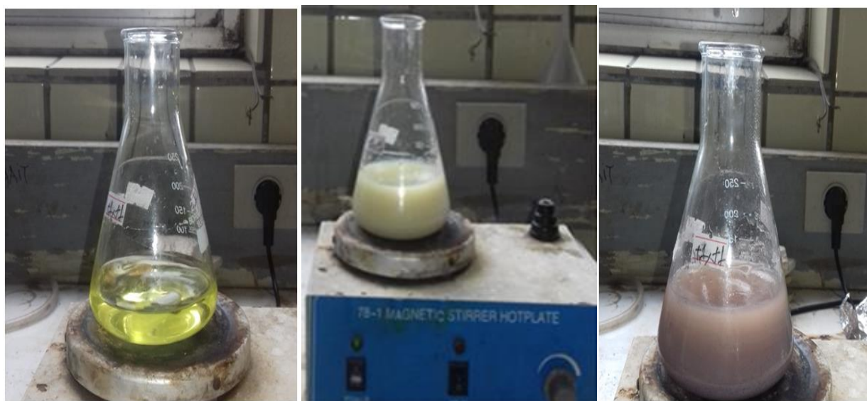
Figure D3: chloride test of salt samples using \text{AgNO}_3 and \text{KCr}_3 indicator
