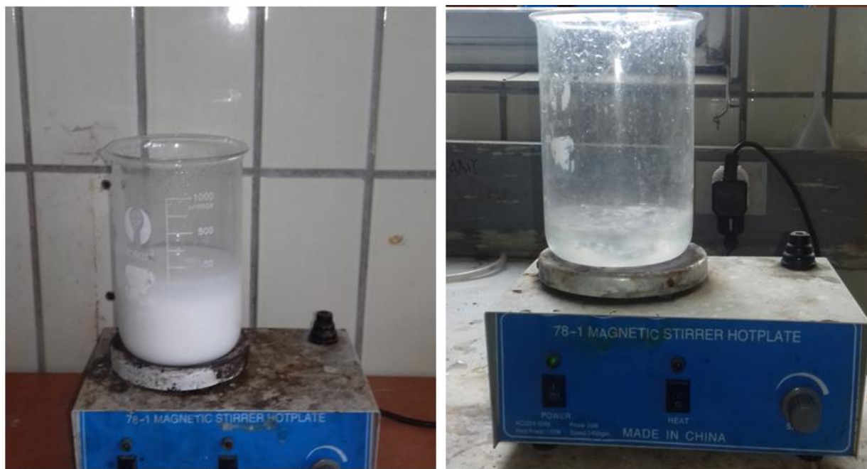
Figure D2: a) gravimetric precipitation of sulphat b) chemical treatment purification.
