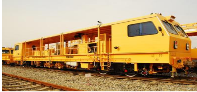
Figure 2.6– Dynamic Track Stabilizer [Unitedindustrial, 2013]
