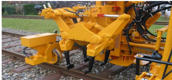
Figure 2.4– Tamping Machine [Plasser and Theurer, 2013]
