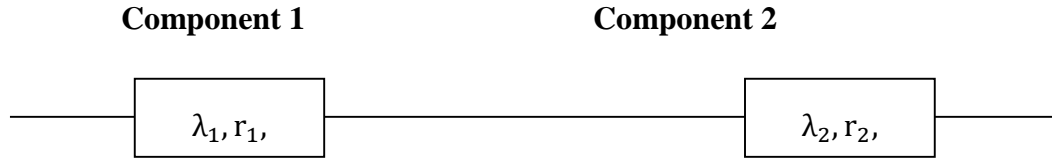
Figure 5 Mathematical Model for two components in Series
