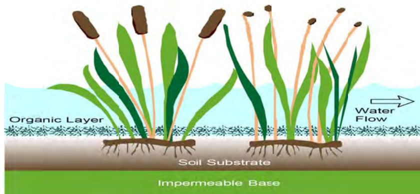
Figure 2.3 Surface Flow Constructed Wetland
