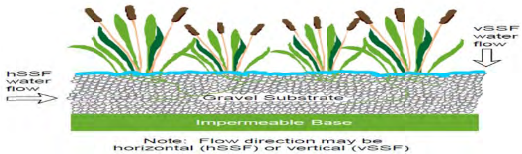
Figure 2.4 Subsurface Flow Constructed Wetland
